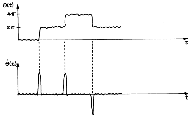
Figure 7. Input and Output of Ideal FM Discriminator
