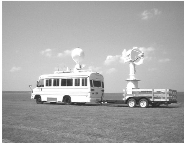
A key area being addressed by the RTPS IV project is remote site support. Pax River supports detachments aboard aircraft carriers and land-based sites with personnel and portable telemetry handling systems. As part of RTPS IV, the portable systems will be 100 percent compatible with the central system at Pax River. This will dramatically reduce preparation time needed for taking equipment into the field and will provide the same advanced features as the home system.
