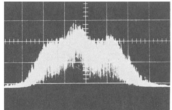
3B. Abnormally Aligned System Noise Spectrum
