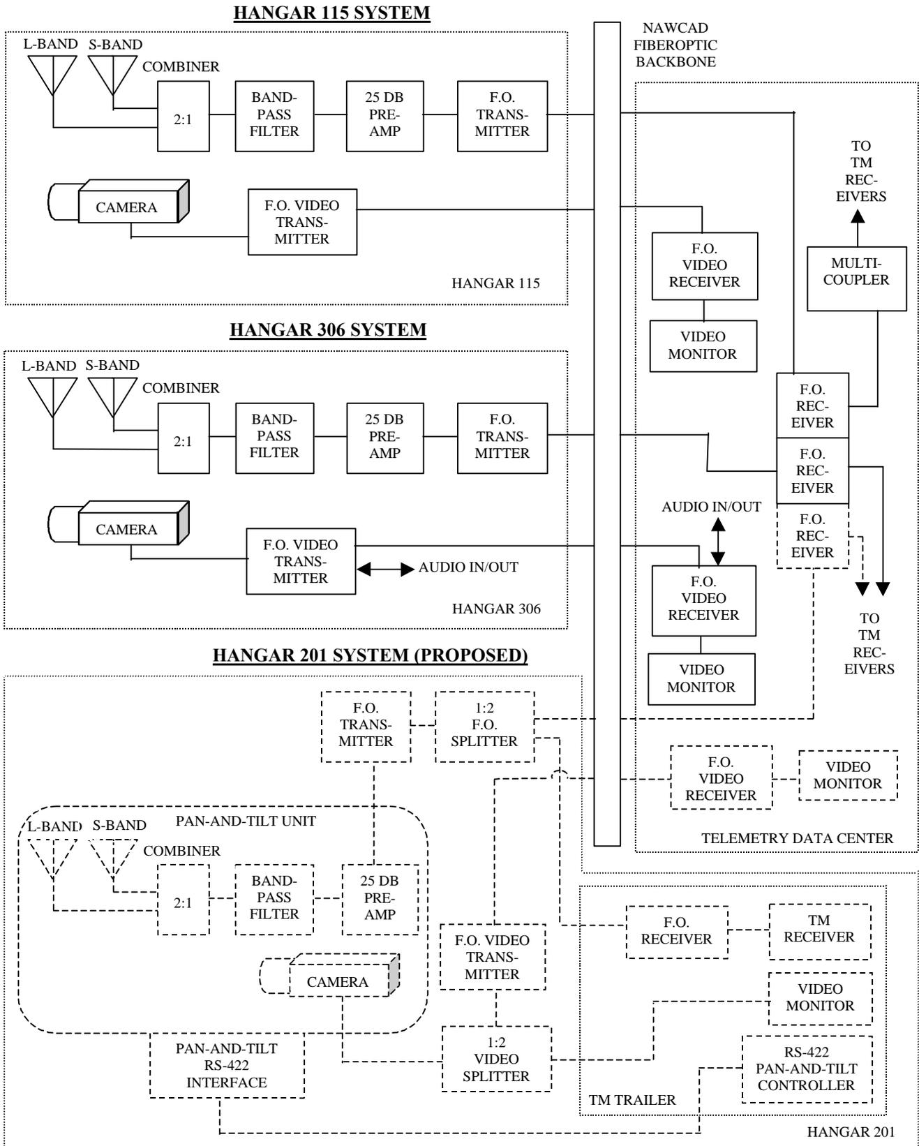
Figure 3. Total System Configuration
