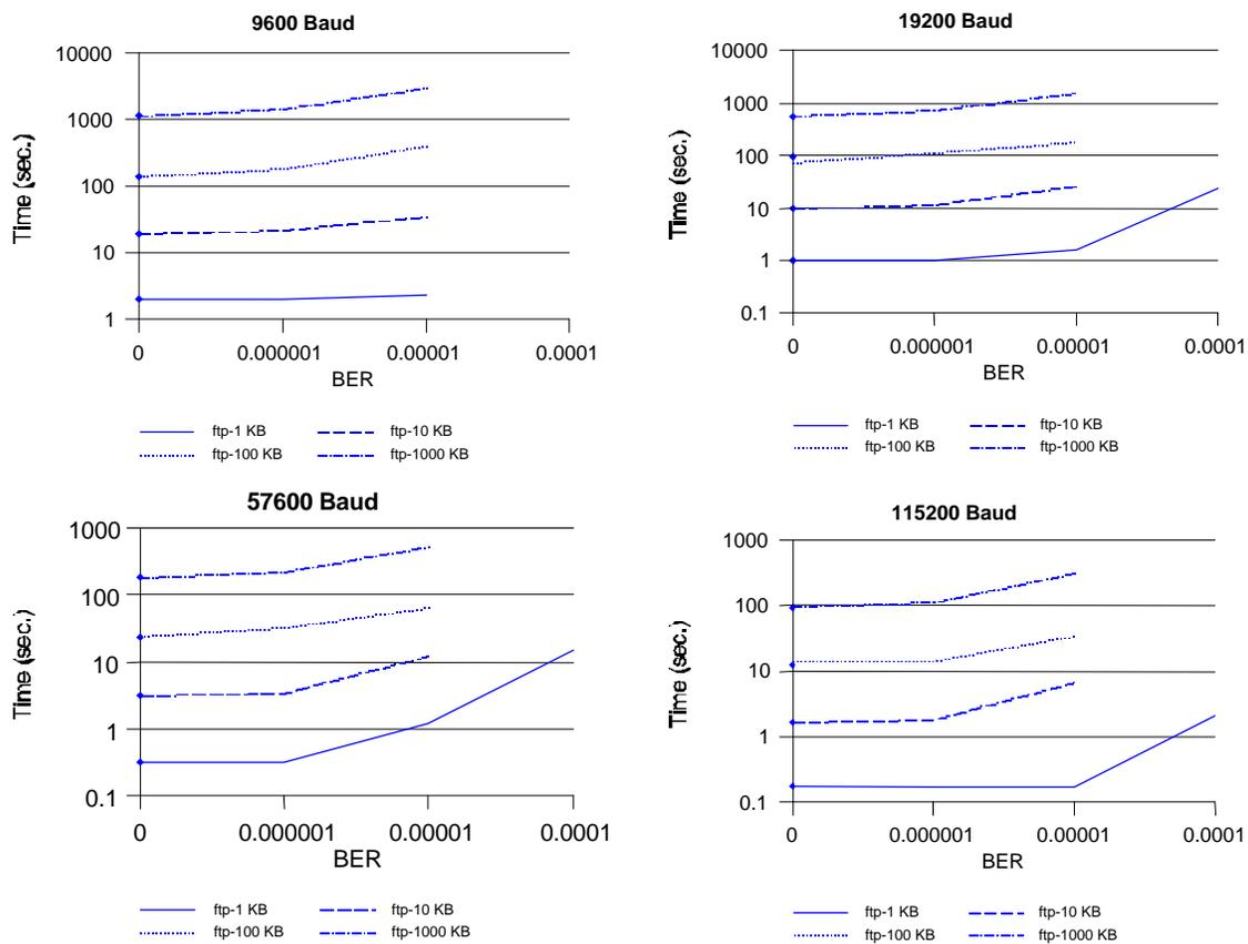
**Figure 1 - File transmission time results using the FTP service as a function of BER and baud rate.**
