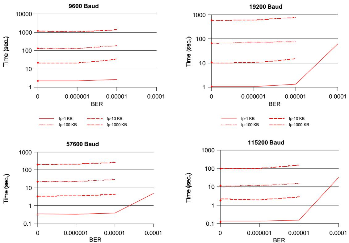
**Figure 2 - File transmission time results using the FP service as a function of BER and baud rate.**
