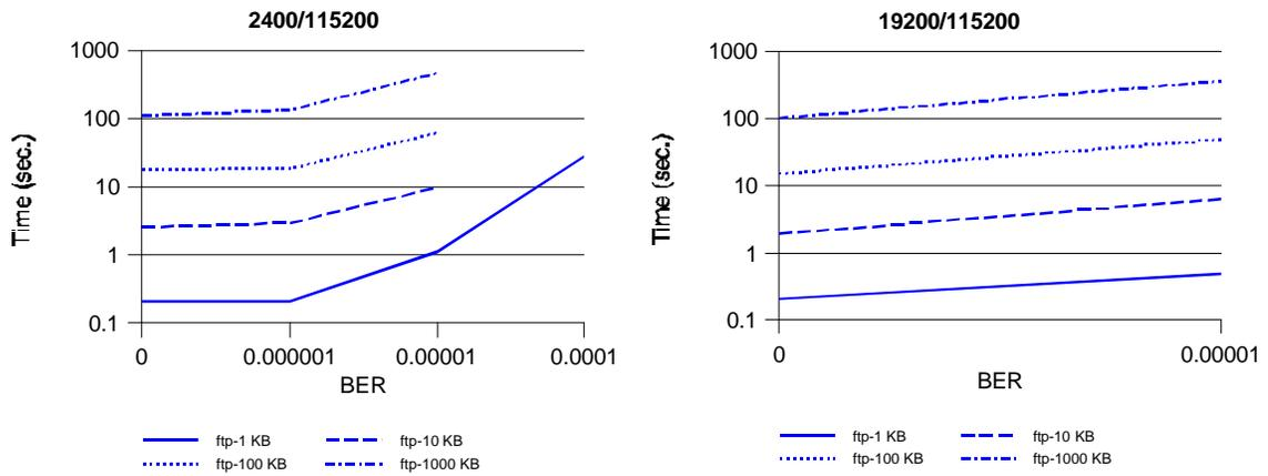
**Figure 3 - Unbalanced transmission test time for the FTP service as a function of file size and BER**
