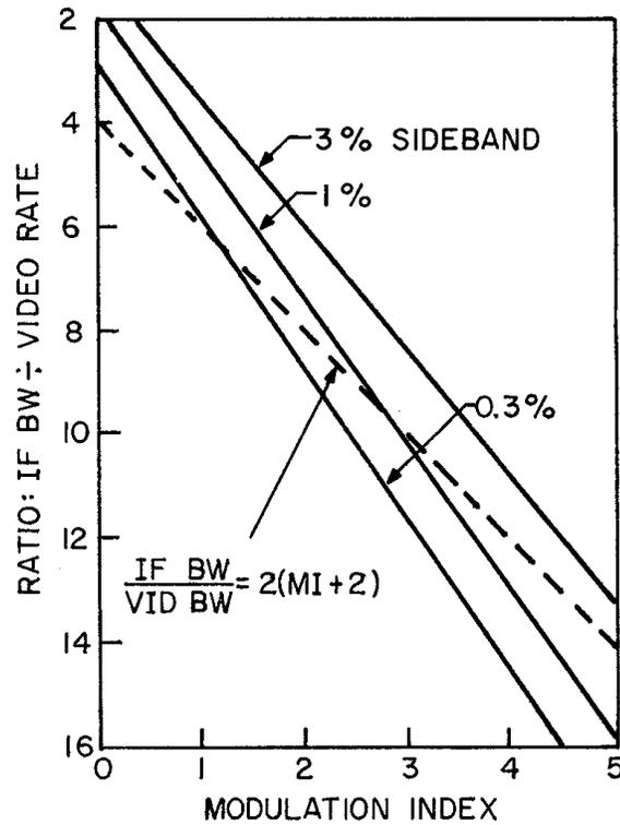
**Fig. 5. IF Bandwidth to Video Rate Ratio**
