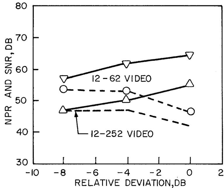
**Fig. 4. NPR, SNR vs Transmitter Deviation For Two Video Bandwidths**
