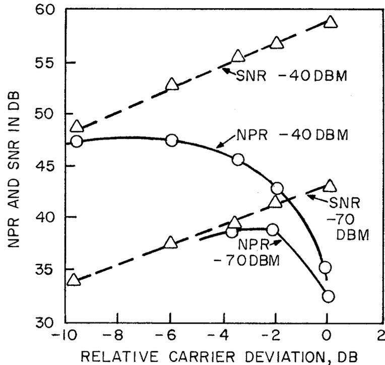
**Fig. 2. NPR and SNR vs Carrier Deviation.**
