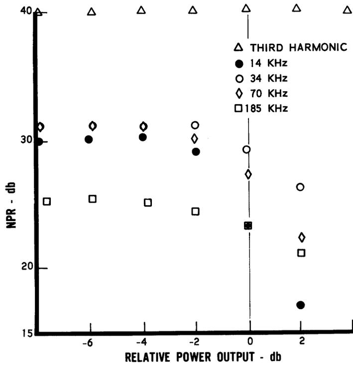
FIGURE 5 NPR TEST DATA AS A FUNCTION OF OUTPUT POWER WITH INPUT POWER CONSTANT
