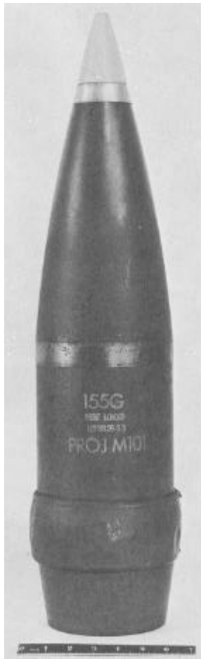
Fig. 23 - UHF TM in Ogive of a 55 Mm Projectile
