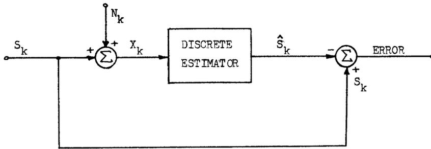
**FIGURE 1. Discrete estimation system model.**
