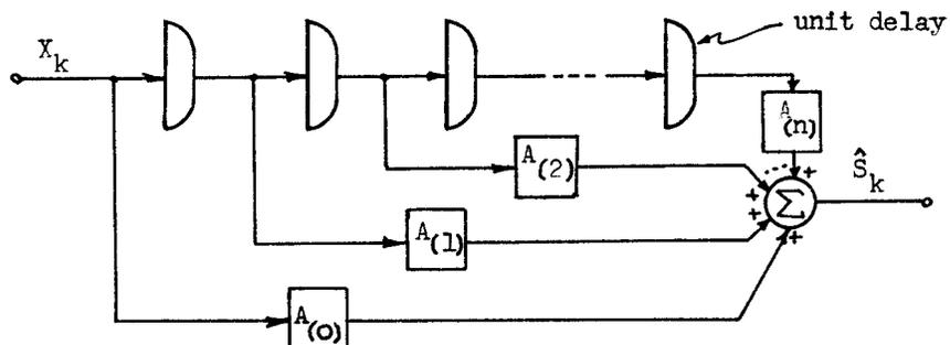
**FIGURE 3. Model of the discrete linear nonrecursive estimator.**
