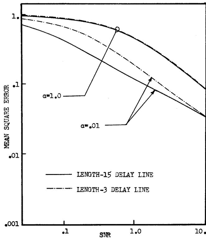
FIGURE 4. Mean square error versus SNR for the discrete linear non-recursive filters of lengths 3 and 15 with  $v=1.0$ .
