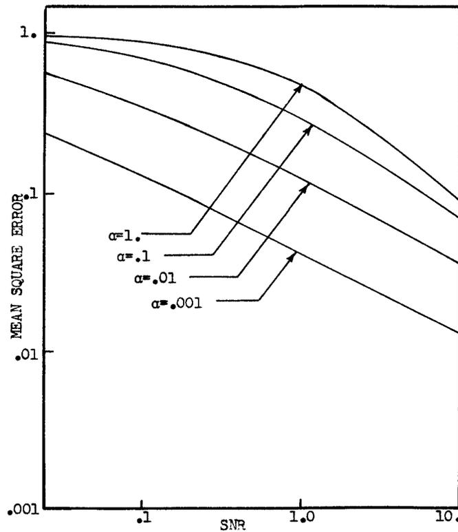
**FIGURE 2. Mean square error versus SNP for the optimum realizable discrete Wiener-Hopf filter, where  $v=1.0$ .**
