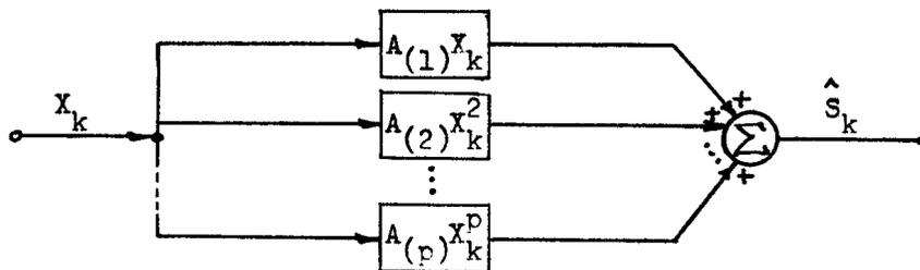
FIGURE 5. The model of the discrete nonrecursive Type estimator.
