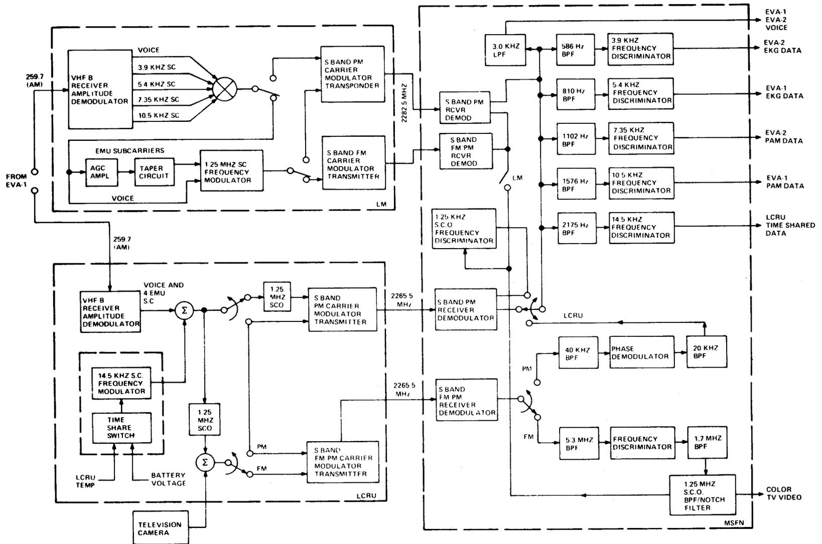
**Figure 6. Down-link Communications system, EVCS/LCRU/MSFN and LM/LCRU/MSFN**
