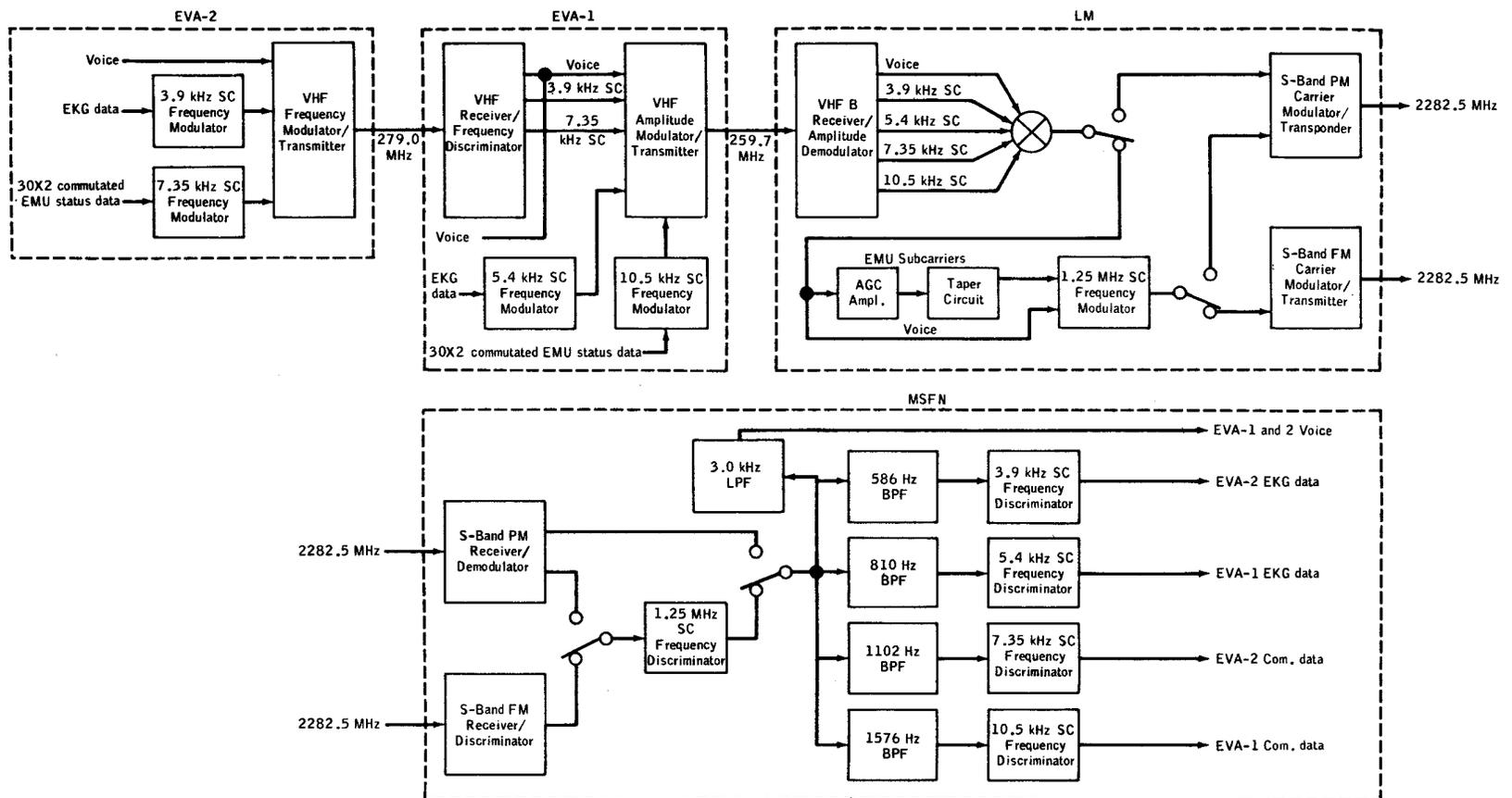
**Figure 2. Down-link EVA-to-MSFN Communications System Configuration (Dual Mode)**
