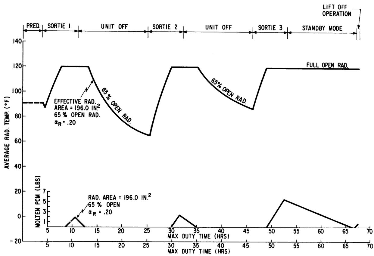
Figure 11. Average Radiator Temperature Vs Maximum Duty Time with a 20° Sun Angle Start and Hot Traverse
