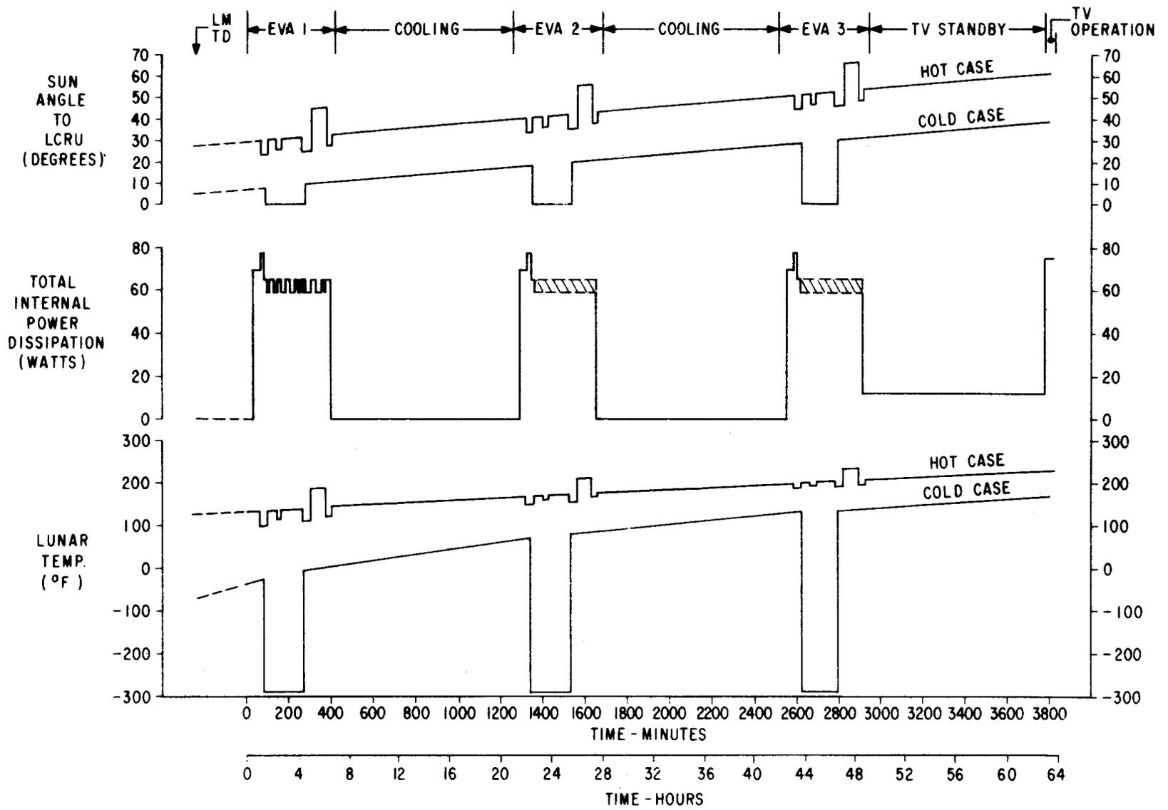
Figure 4. LCRU Timeline No. 1 (Including Dissipation)
