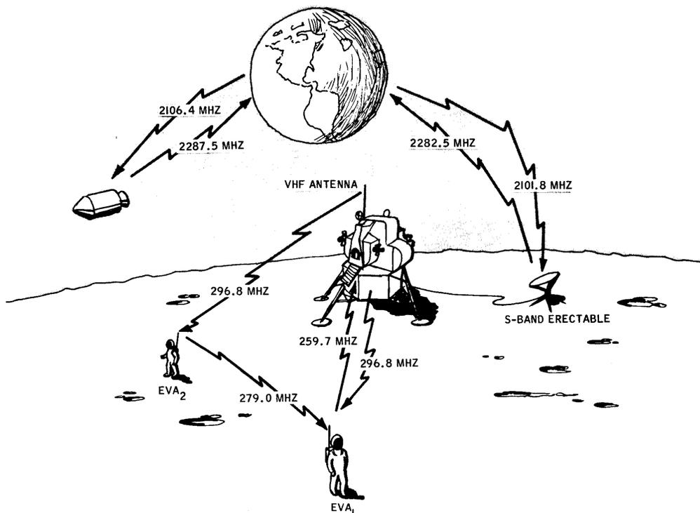
**Figure 1. EVA.-to-MSFN Relay Communications System**
