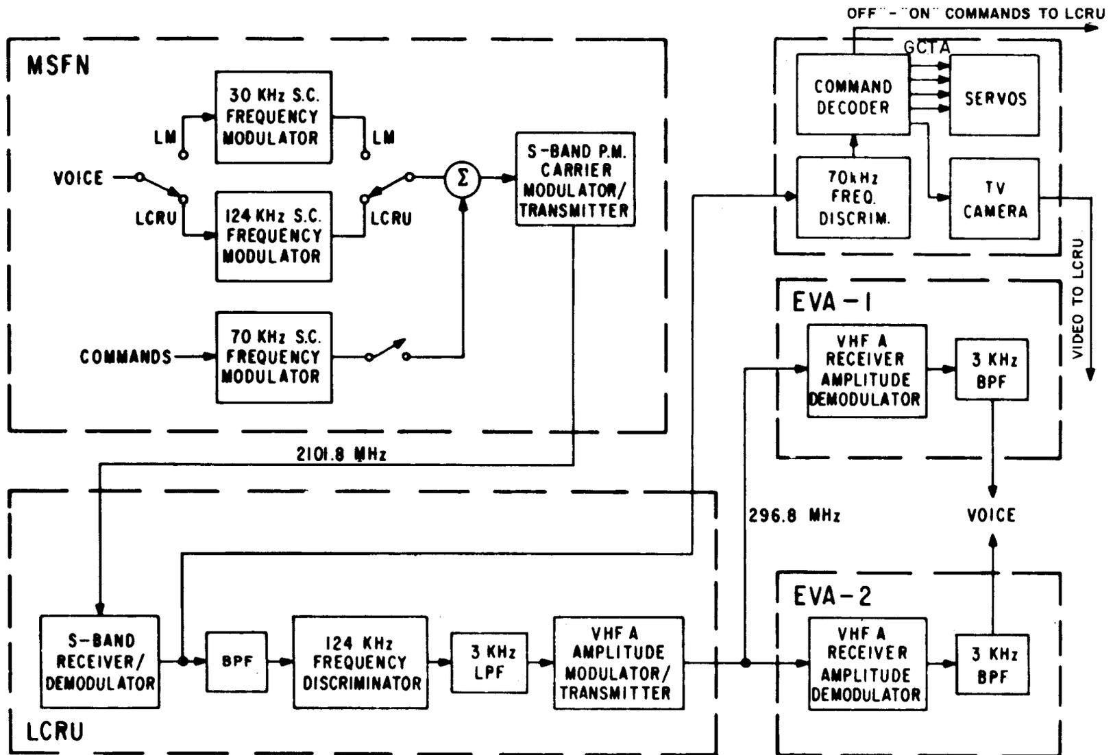
Figure 7. Up-link MSFN/LCRU/EVA.-1/EVA.-2 Communications System
