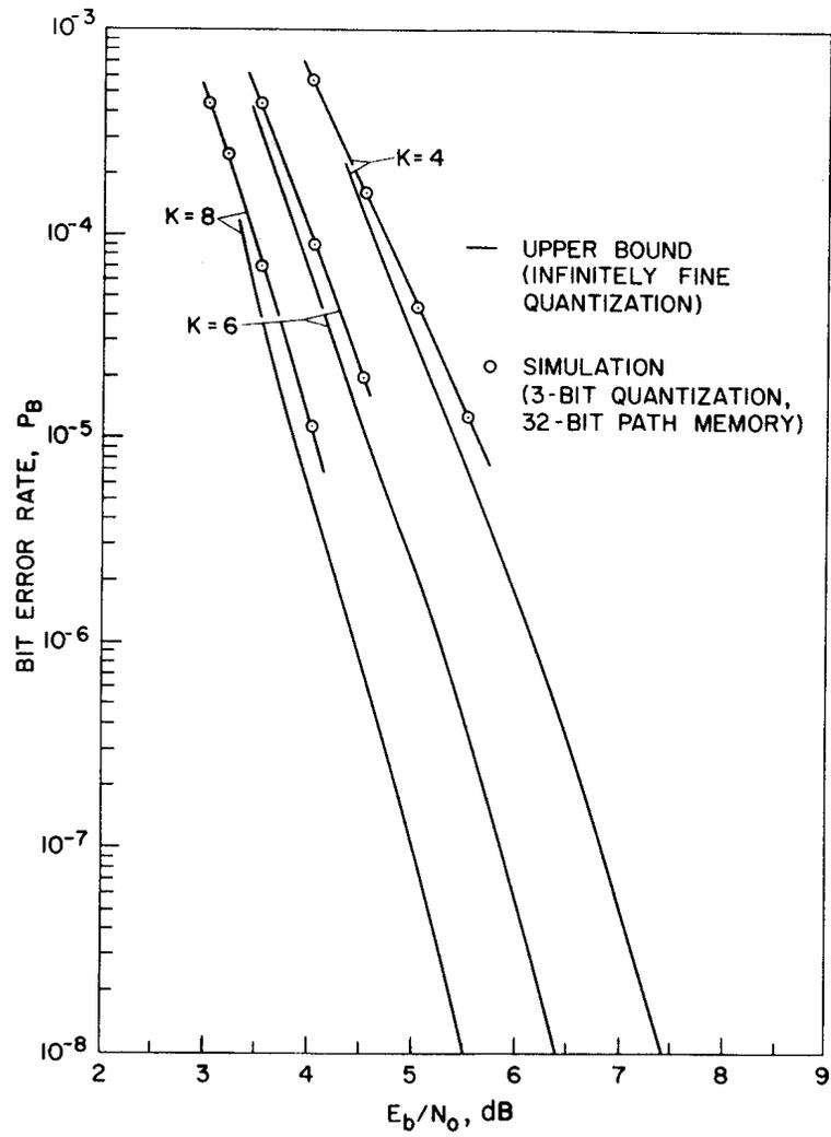
**Fig. 1 - Bit Error Rate vs.  $E_b/N_0$  for Rate 1/2 Viterbi Decoding.**
