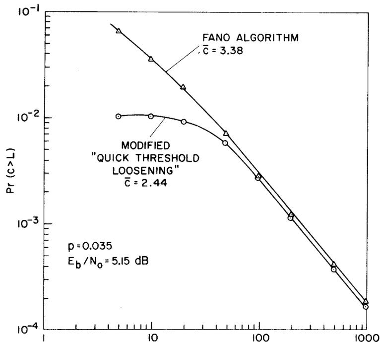
**Fig. 3 - Distribution of Computation Comparison for the Standard Fano Algorithm and the Modified "Quick Threshold Loosening" Sequential Decoders.**
