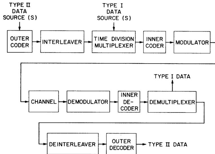
**Fig. 2 - Coding for Data of Varying Error-Rate Requirements.**
