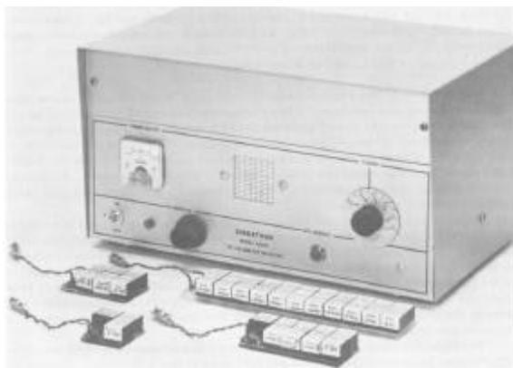
Two channel FM-FM telemetry transmitter for ECG and ZPG on separate IRIG sub-carriers, and one transmitting carrier in the 215-260 MHz band. (Courtesy of Bio-Sentry Telemetry, Inc., Torrance, California.)
