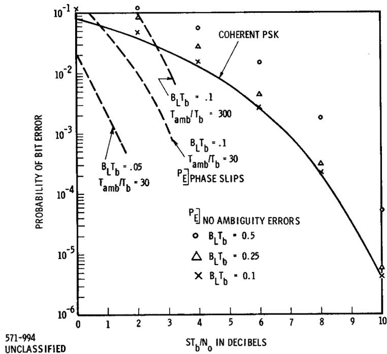
**Figure 4. Biphase Performance with Suppressed Carrier Tracking - Ambiguity Resolution on Carrier Component**
