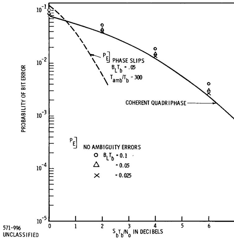
**Figure 5. Quadriphase Performance with Suppressed Carrier Tracking - Ambiguity Resolution on Carrier Component**
