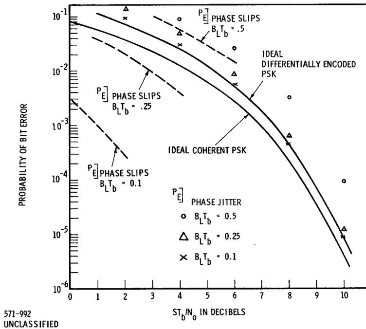
**Figure 3. Differentially Encoded Biphase Performance with Suppressed Carrier Tracking**
