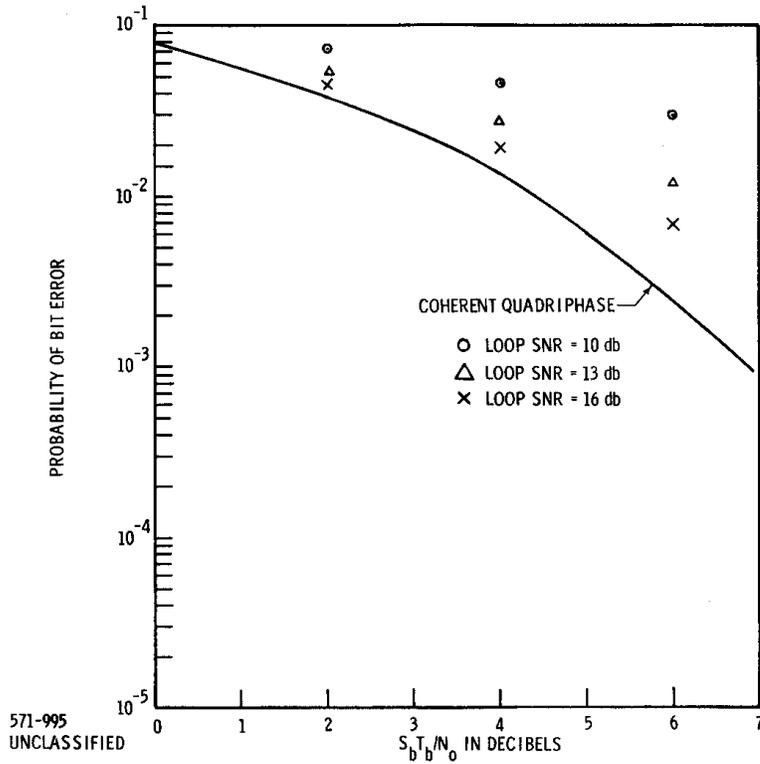
**Figure 2. Quadriphase Performance With Carrier Tracking**
