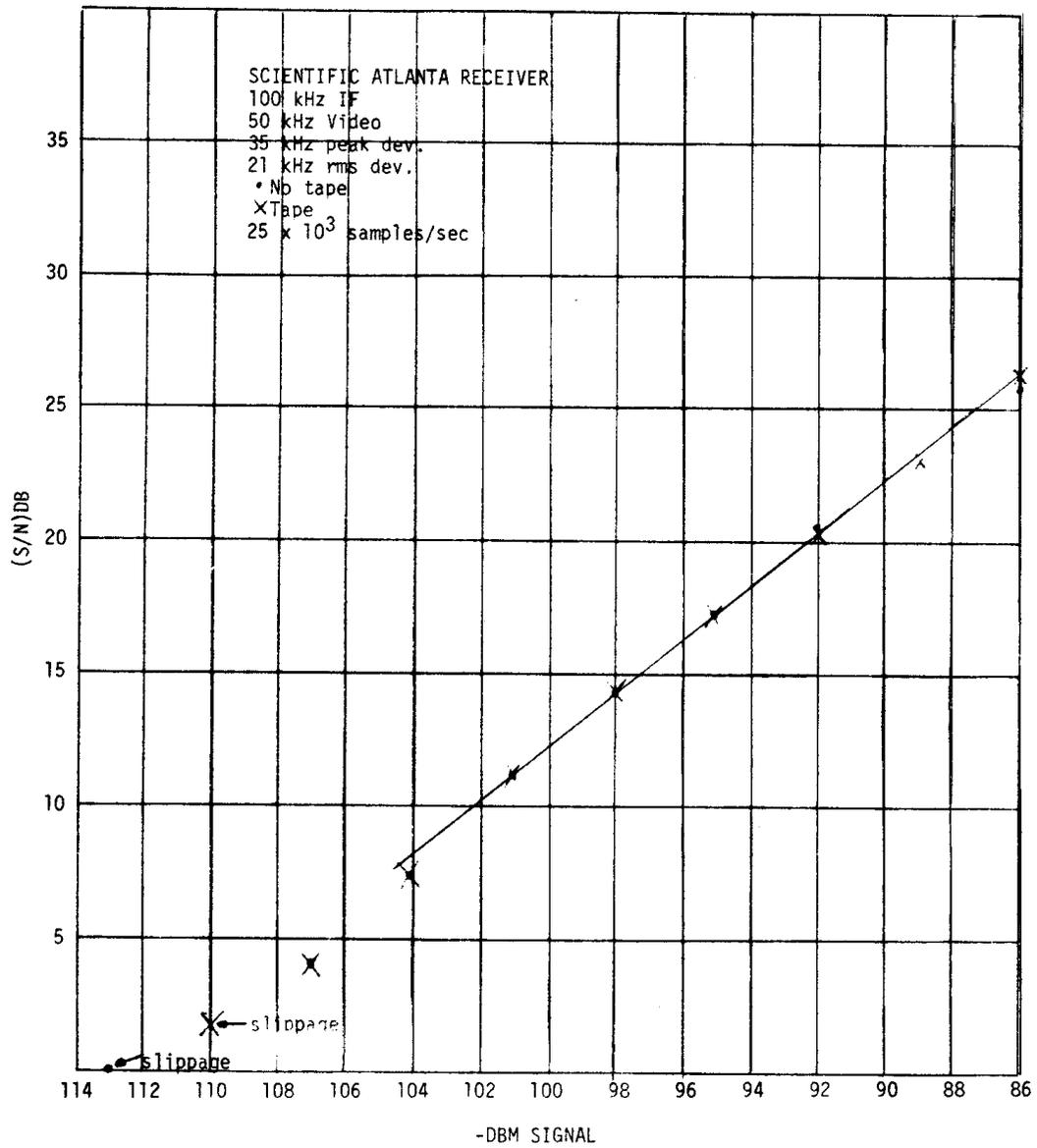
**FIGURE 4. OUTPUT RMS (S/N) IN DB VERSUS INPUT SIGNAL POWER IN DBM**
