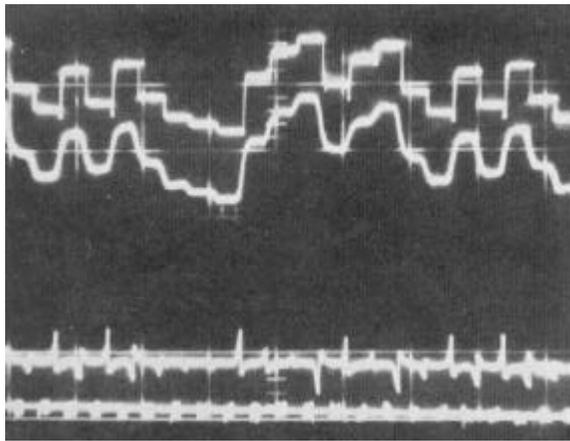
**FIGURE 6A. TAPE OUTPUT WITH -56 DBM INPUT TO RECEIVER**
