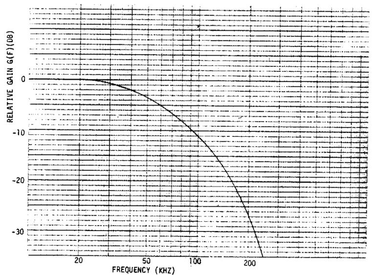
**FIGURE 8. VIDEO OUTPUT RELATIVE GAIN CHARACTERISTIC**
