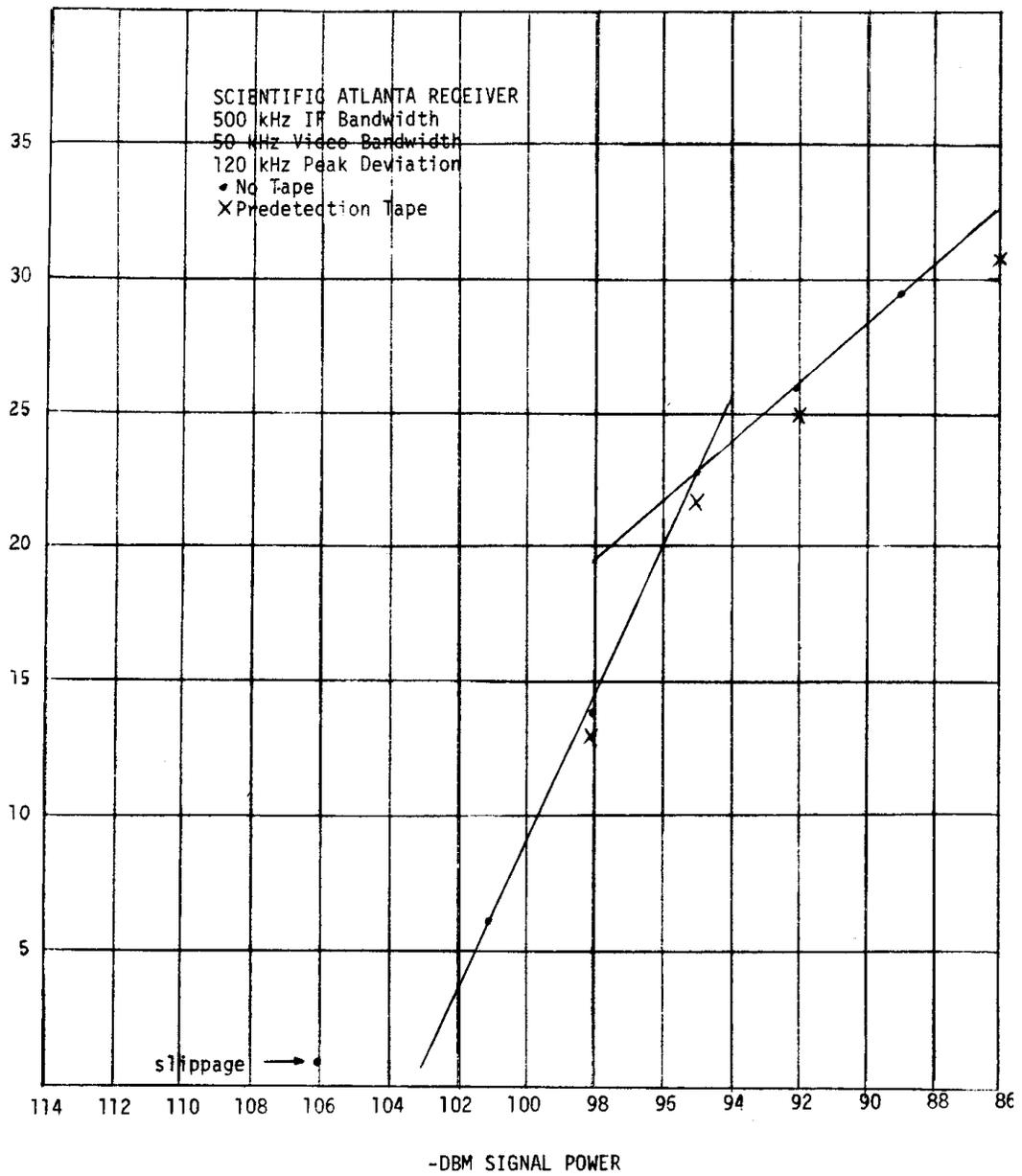
**FIGURE 3. OUTPUT RMS (S/N) IN DB VERSUS INPUT SIGNAL POWER IN DBM**
