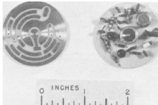
Fig. 3 - Modulator, 75-MHz Crystal oscillator, and Power Amplifier
