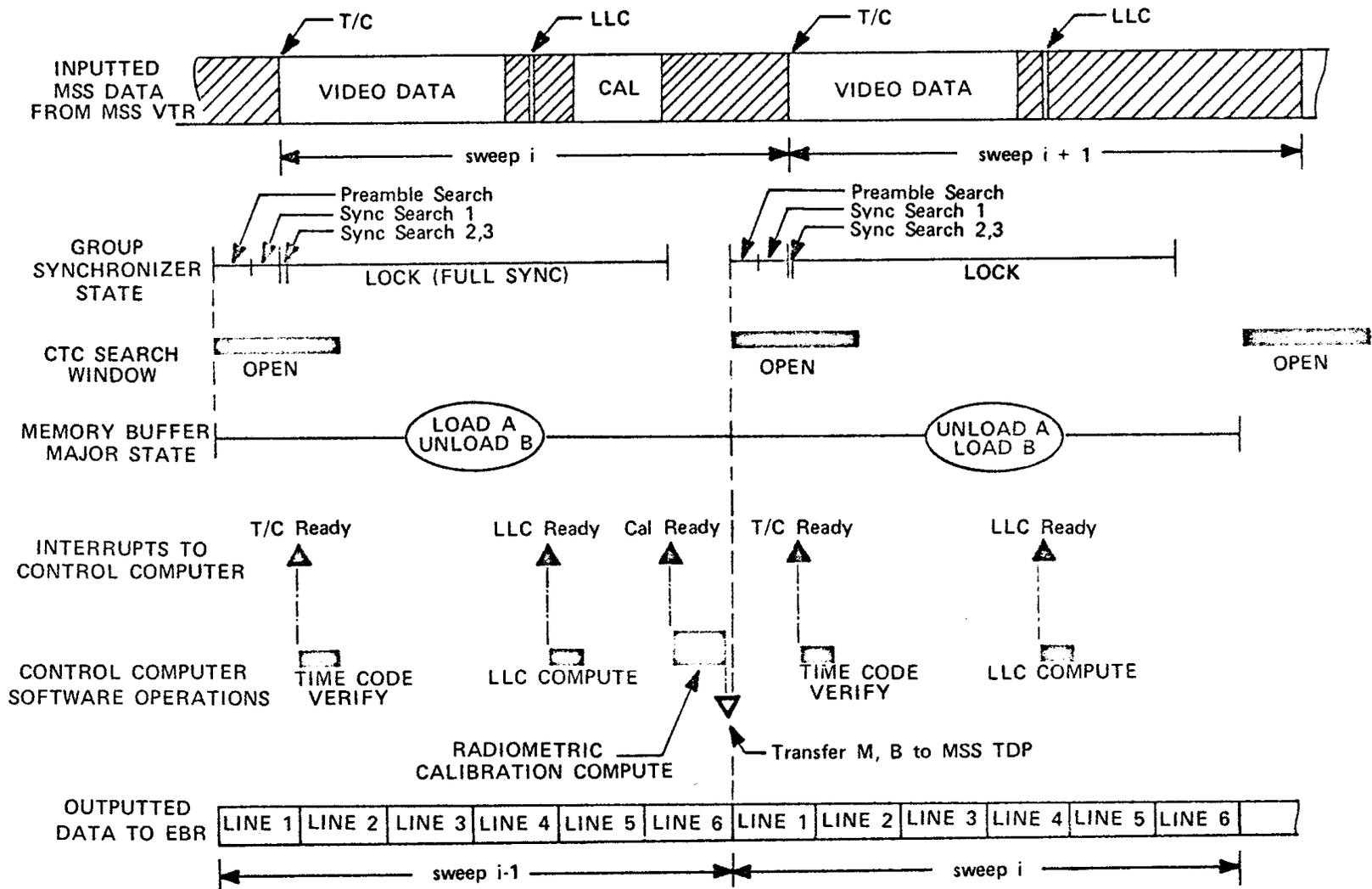
**Fig. 6 - MSS TDP Operational Timeline (MSS VTR to EBR Mode.)**
