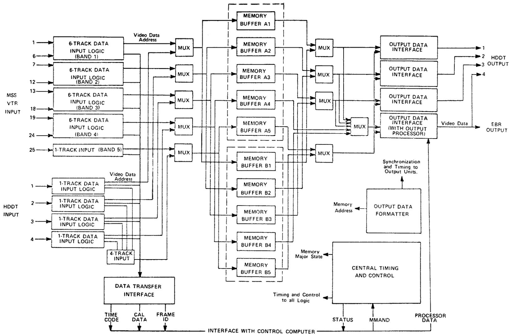
**Fig. 2 - MSS-TDP Block Diagram.**
