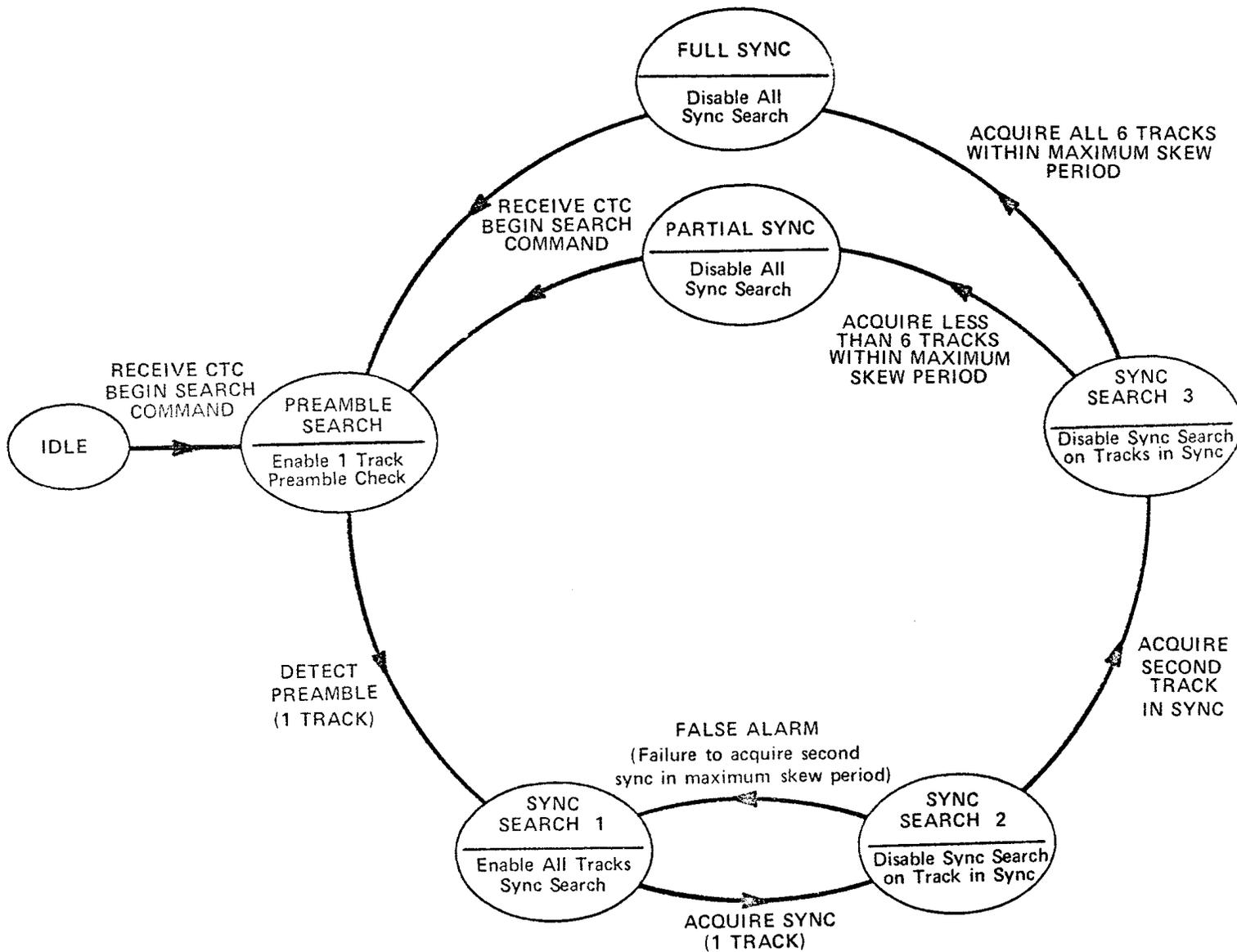
**Fig. 4 - Group Synchronizer State Transition Diagram**
