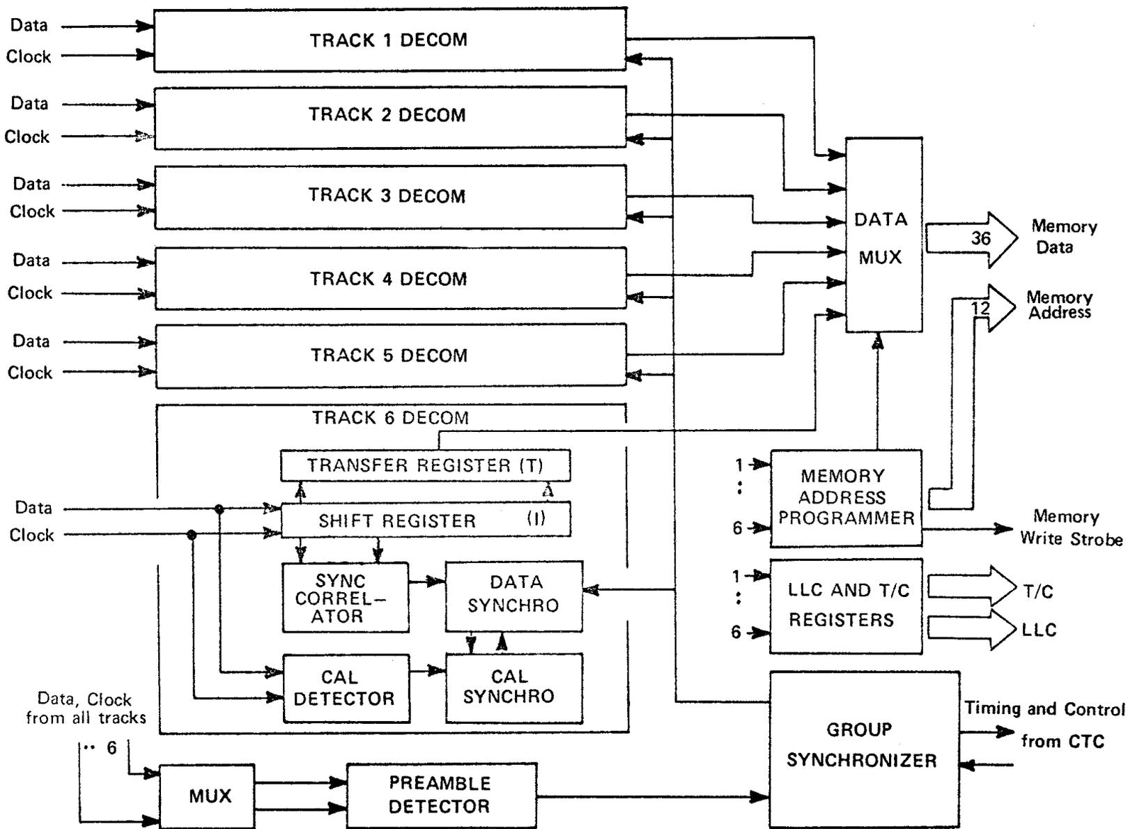
**Fig. 3 - MSS TVR 6-Track Input Decommutator/Synchronizer.**
