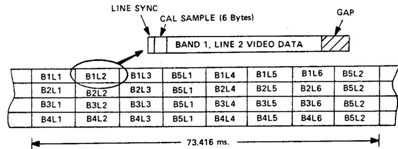
Fig. 1 - Multispectral Scanner Data Flow and Formats.
