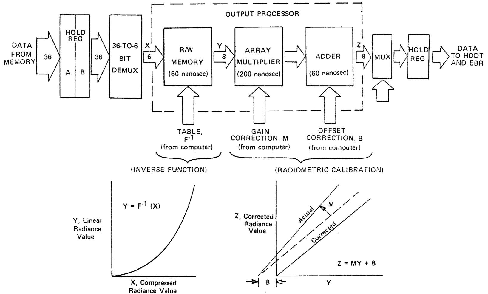
**Fig. 5 - Processor Operations and Hardware Configuration.**
