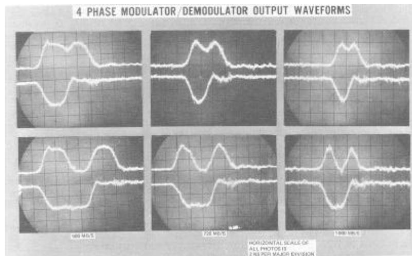
**Figure 9. Demodulator Output Waveforms**
