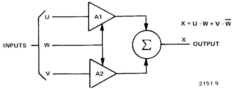
**Figure 3. Functional Arrangement for the Multiplier/Signal Switch**
