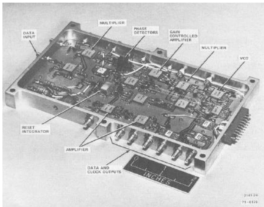
Figure 16. 200 MB/S Bit Synchronizer and Matched Filter
