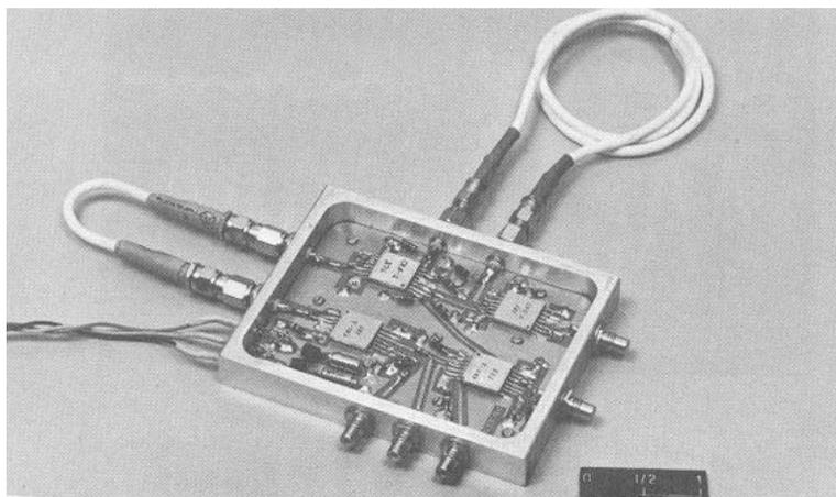
**Figure 7. Photograph of the 1000 MB/s PN Generator**
