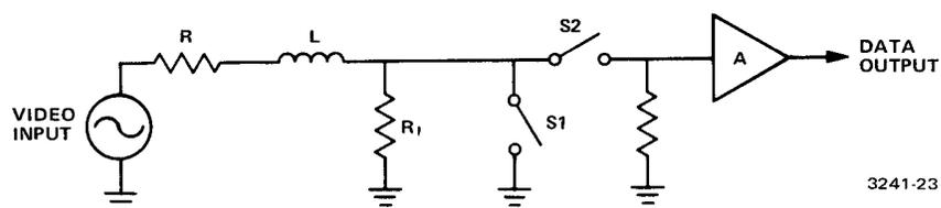
Figure 17. Simplified Diagram of the Reset Integrator
