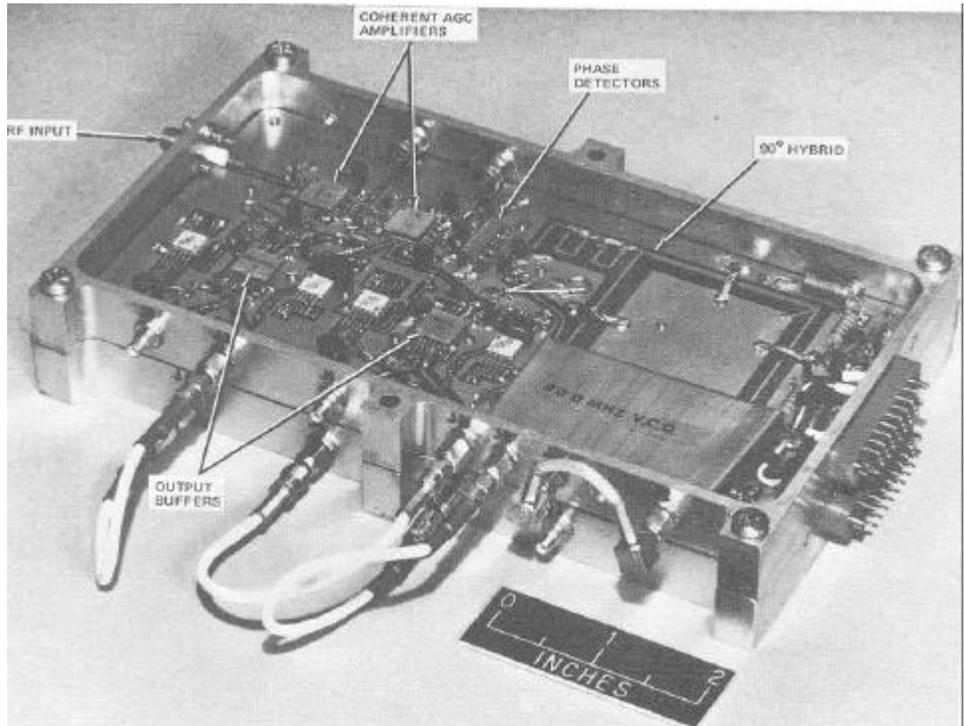
**Figure 14. 4-Phase Demodulator and Phase Detector**
