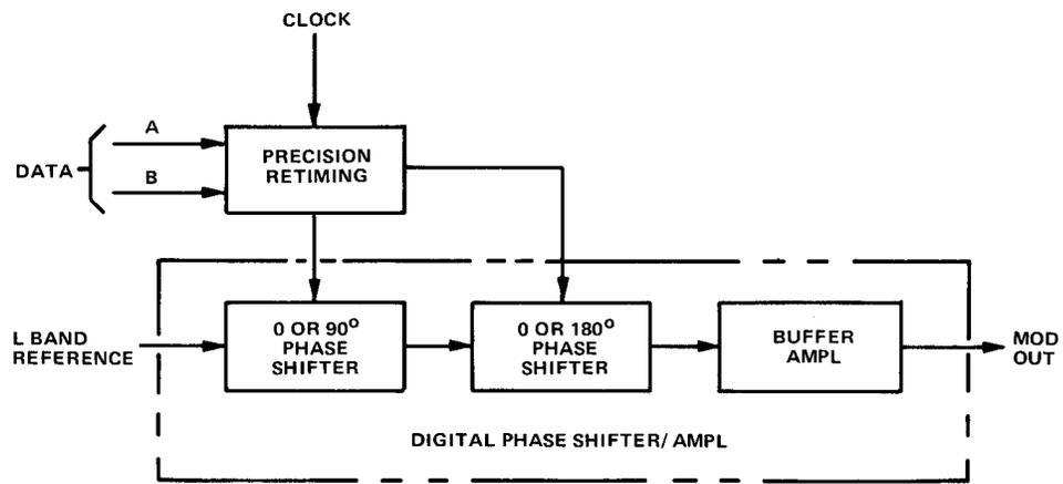
**Figure 8. Modulator Subsystem Functional Block Diagram**
