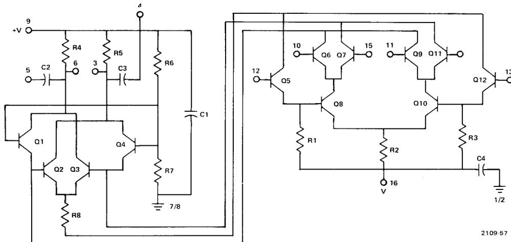
**Figure 2. Schematic of the Multiplier/Signal Switch**
