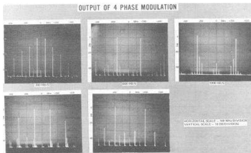
**Figure 10. Spectrum of Modulator**
