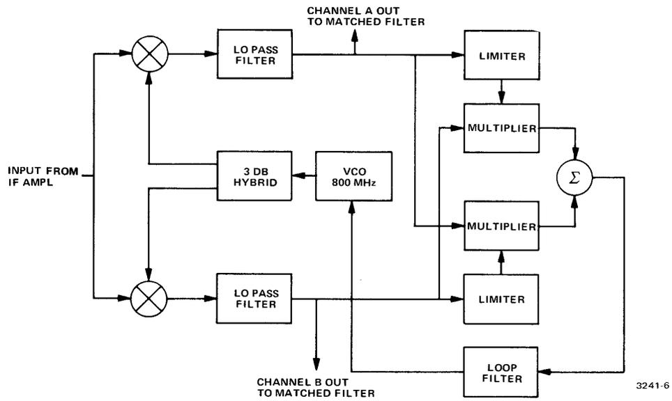
**Figure 13. 4-Phase Demodulator and IQ Loop**
