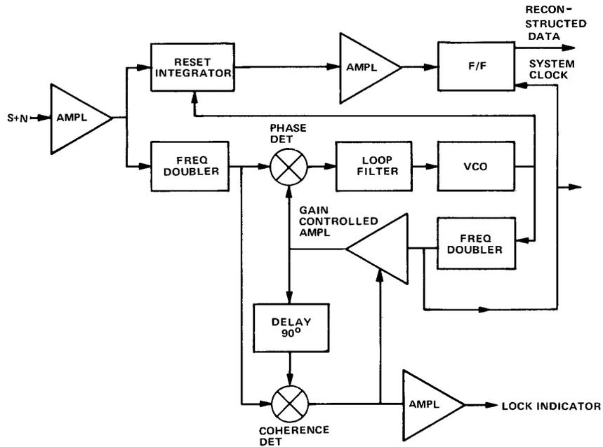
Figure 15. Bit Synchronizer and Matched Filter Block Diagram
