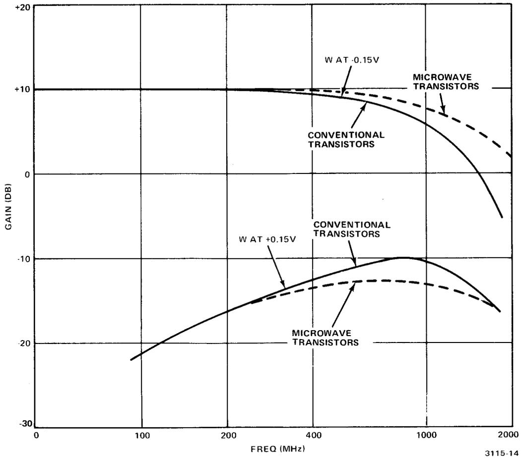
**Figure 4. Frequency Response and Isolation Characteristics of the CRA-II**
