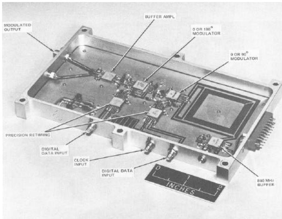
**Figure 12. Quadrphase Modulator and Precision Retiming Module**
