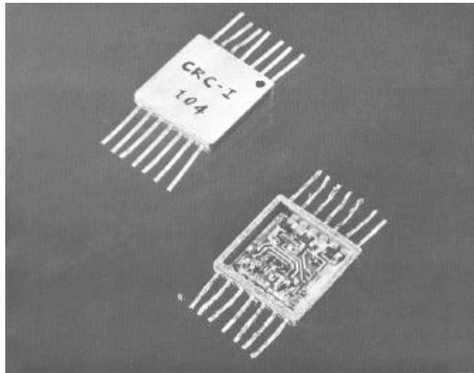
**Figure 1. Switch Constructed on a Sapphire Substratae**
