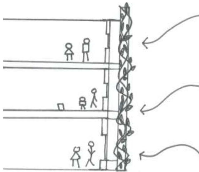
*Figure 9 Vertical Shading Blades with Vegetation for Natural Ventilation. Illustrated by Ambar A. Gardner.*
