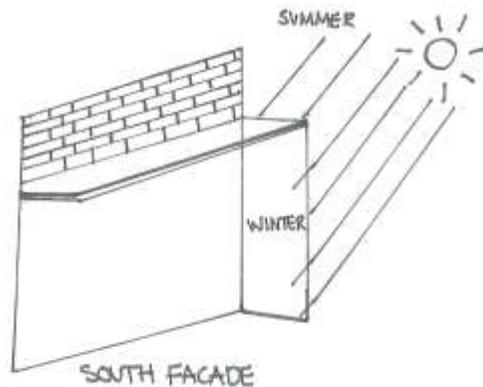
*Figure 6 Vertical Fin with a Horizontal Overhang. Illustrated by Ambar A. Gardner.*
