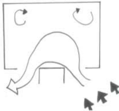
*Figure 15* Example of air flow intercepting wing walls (Source: Arens 1989 Document pg. 35).
