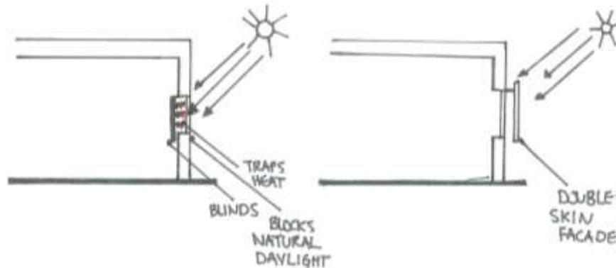
Figure 14 Blinds vs. Double Skin Façade for Passive Cooling. Illustrated by Ambar A. Gardner.
