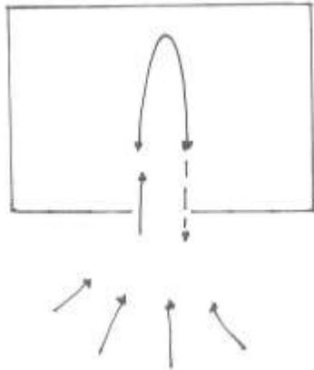
*Figure 16 One Opening on the Windward Wall. Illustrated by Ambar A. Gardner.*
