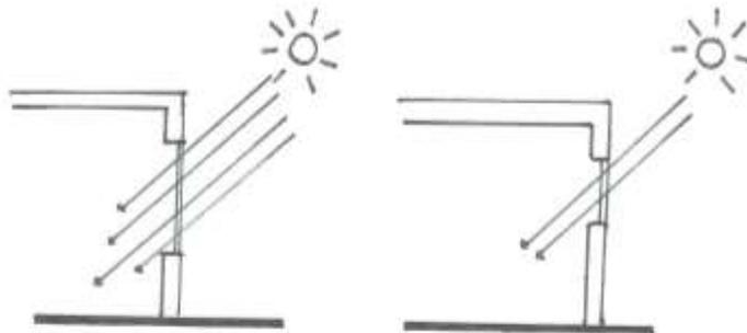
*Figure 3 Solar Gain Entering the Space in Response to the Size of Window. Illustrated by Ambar A. Gardner.*
