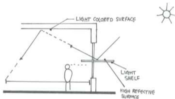
*Figure 12 Secondary and Tertiary Daylight. Illustrated by Ambar A. Gardner*
