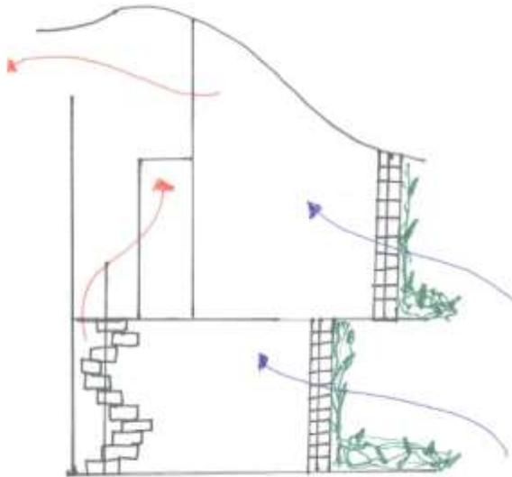
*Figure 18 Cross Ventilation. Illustrated by Ambar A. Gardner.*
