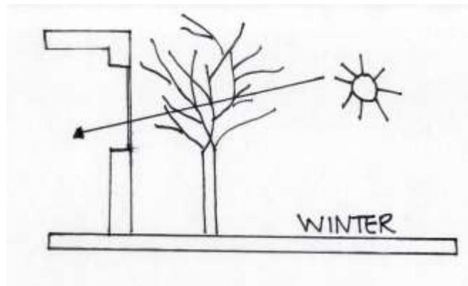
Figure 11 Deciduous Tree Used for Passive Heating in the Winter. Illustrated by Ambar A. Gardner.
