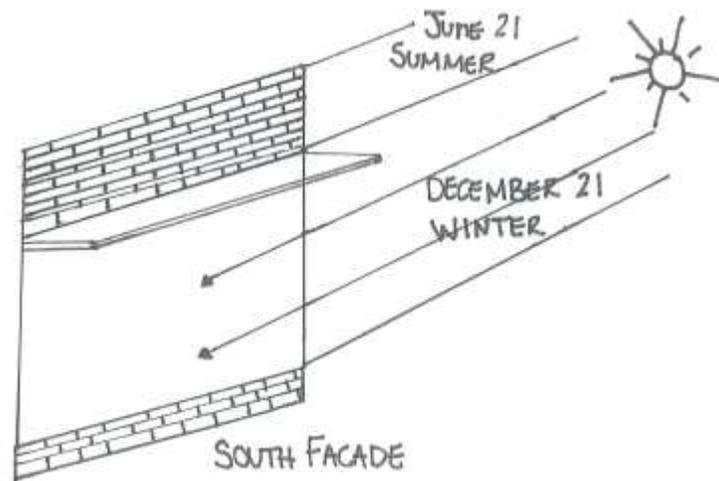
Figure 4 Horizontal Overhang. Illustrated by Ambar A. Gardner.
