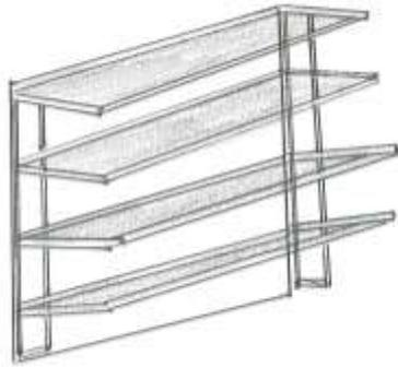
*Figure 7 Horizontal Louvers. Illustrated by Ambar A. Gardner*
