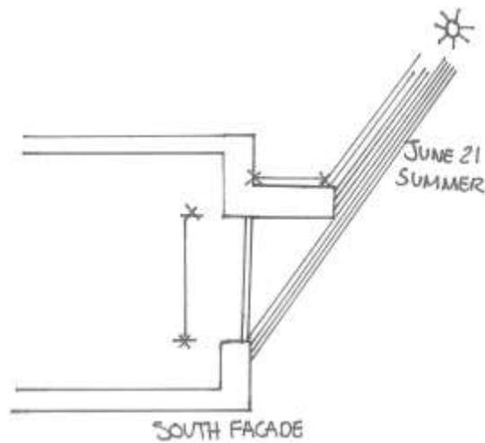
Figure 5 Horizontal Overhang Section View. Illustrated by Ambar A. Gardner.
