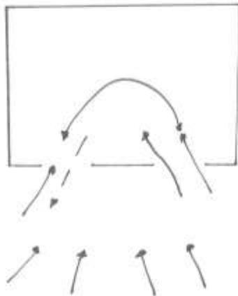
*Figure 17 Two Openings on the Same Wall to Better Distribute Airflow. Illustrated by Ambar A. Gardner.*
