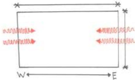
*Figure 2 Orientation of Building Elongated in the East-West Direction to Minimize Heat Gain. Illustrated by Ambar A. Gardner.*
