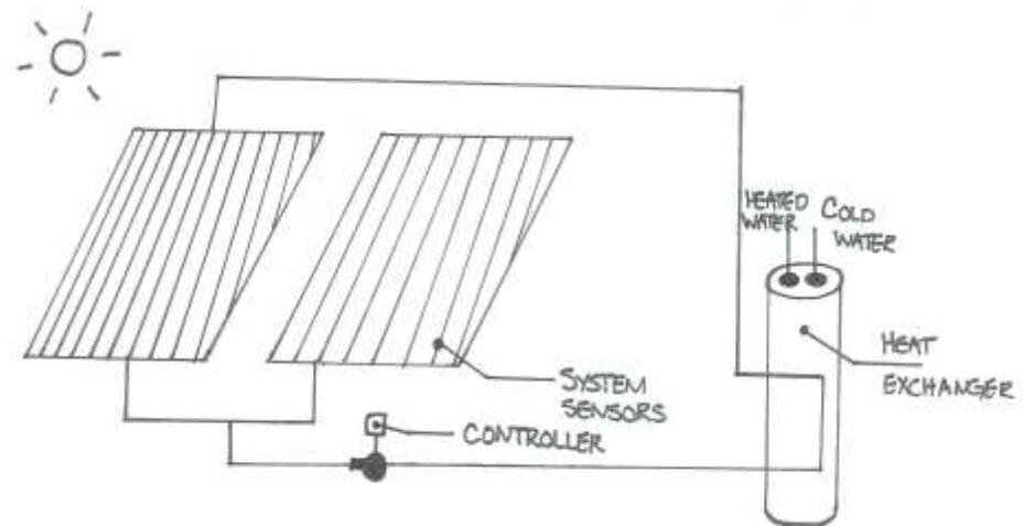
*Figure 22 Solar hot water collector system. Illustrated by Ambar A. Gardner*
