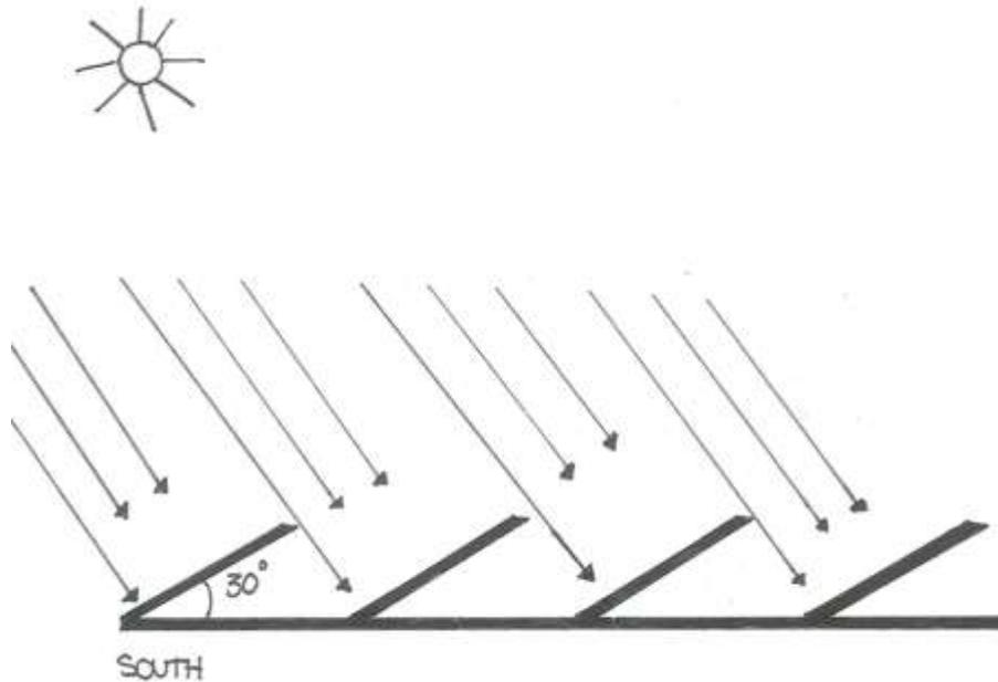
*Figure 21* Appropriately calculated placement of photovoltaics for maximum energy generation. Illustrated by Ambar A. Gardner.
