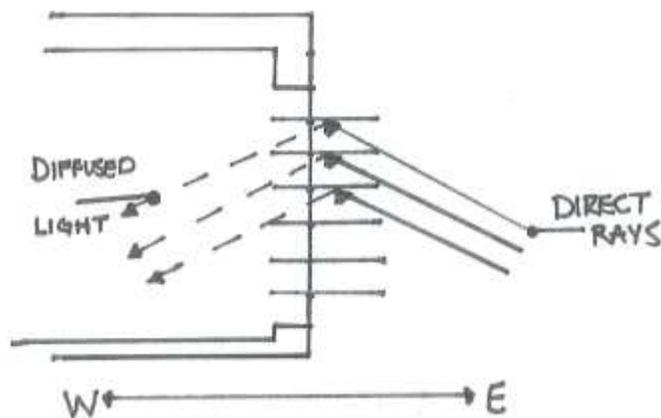
*Figure 8 Horizontal Louvers Plan View. Illustrated by Ambar A. Gardner*
