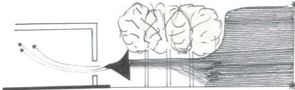
*Figure 13 Evaporative Cooling. Illustrated by Ambar A. Gardner.*
