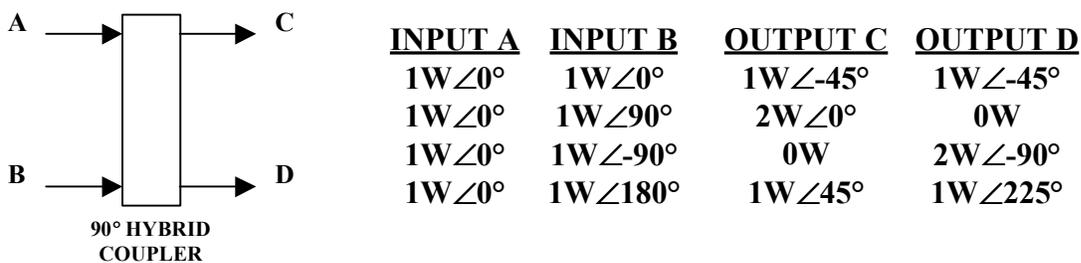
**Figure 1-** Combination of input signals of various relative phases to direct signal to desired output.
