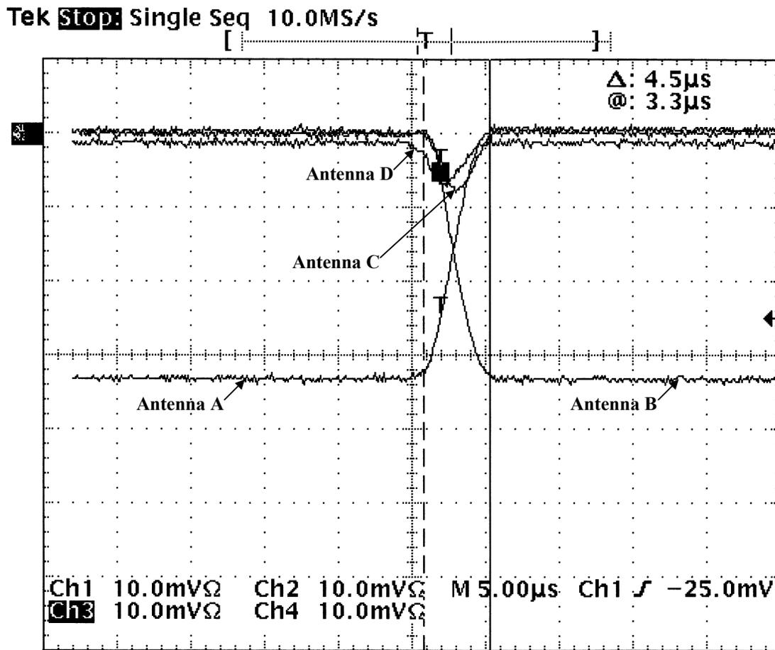
**Figure 5-** Oscilloscope plot of antenna switching time measured using crystal detectors to rectify the RF signals. Note that a negative deflection indicates increasing RF power detected.
