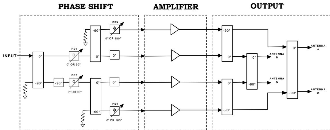
**Figure 3-** Block diagram of the agile RF routing system.
