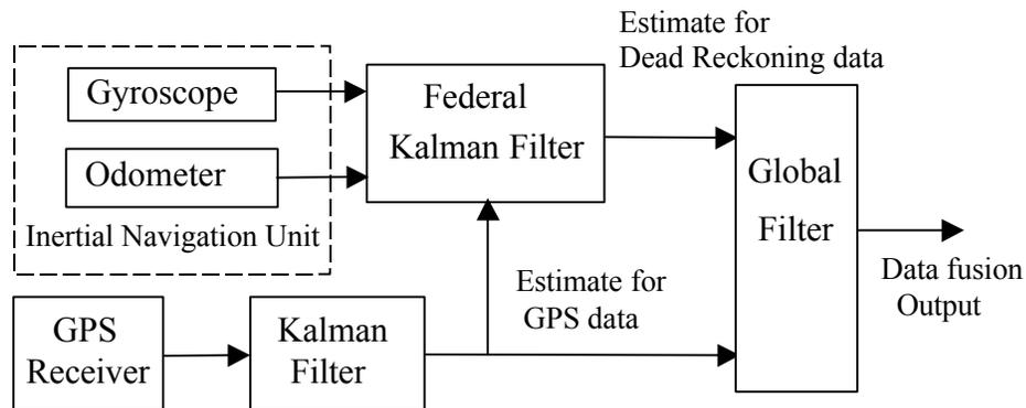
Figure 2. Data fusion process of positioning data
