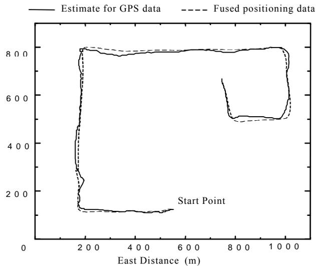
Figure 5. fused positioning data curve
