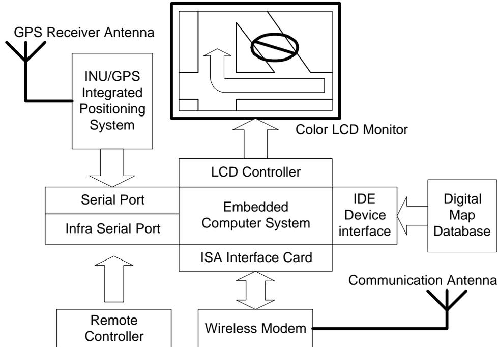
Figure 1. System structure of the AVLNS devising scheme
