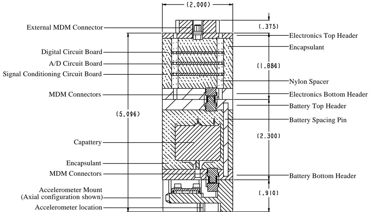
**Figure 3: Cross-section of MinPen Acceleration Recorder**
