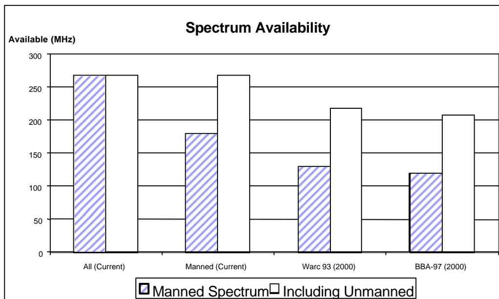
***Figure 1: Current and projected future use of RF spectrum for test and evaluation at Edwards AFB, CA. Spectrum needs increase with advanced avionics systems data requirements at the same time as the available spectrum for test and evaluation decreases due to U.S. Congress reallocation.***
