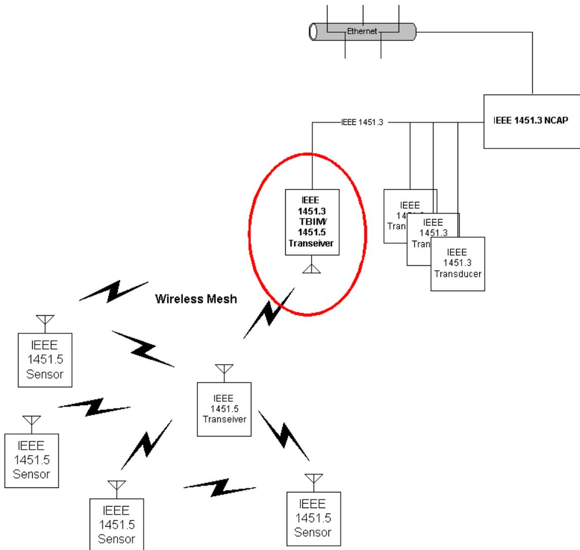
**Figure 4 IEEE 1451.5 Wireless/IEEE 1451.3 Hybrid Transducer System**
