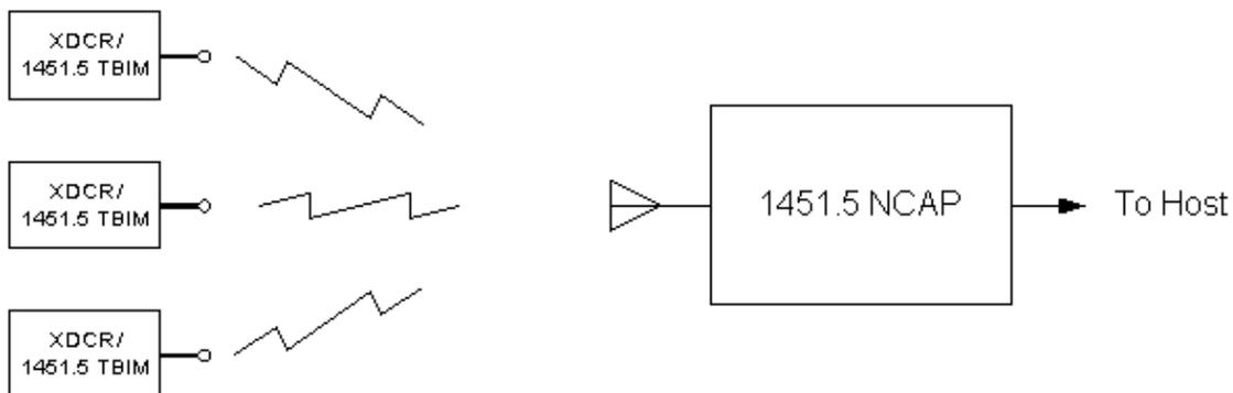
**Figure 2 IEEE 1451.5 Wireless Transducer System**
