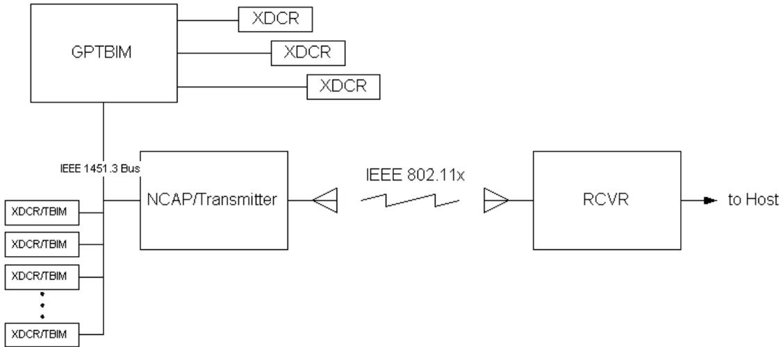
**Figure 1 IEEE 1451.3 Smart Transducer Bus to IEEE 802.11x (Wireless) NCAP**
