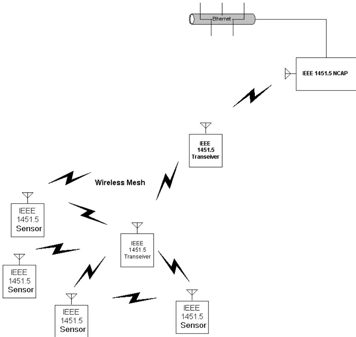
**Figure 3 IEEE 1451.5 Wireless Mesh Transducer System**
