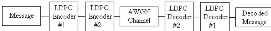
The output of LDPC Encoder #1 consists of the original message bits and the parity bits added by this first stage of encoding. All of these bits are then treated as message bits for the second stage of encoding. Thus, the output of LDPC Encoder #2 consists of the original message bits, parity bits for the original message bits, and parity bits for the output of LDPC Encoder #1. Both encoders are (10,000, 7071) codes and thus the overall rate of this system is 0.5.
