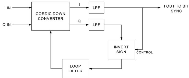
**Figure 7.** Decision Directed Costas Loop with Complex CORDIC Downconverter
