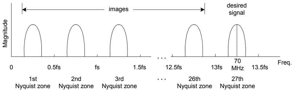
**Figure 4.** Spectral Images Resulting from Undersampling of Analog Waveform
