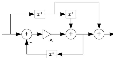
**Figure 5.** Single-stage Half Band Filter Structure
