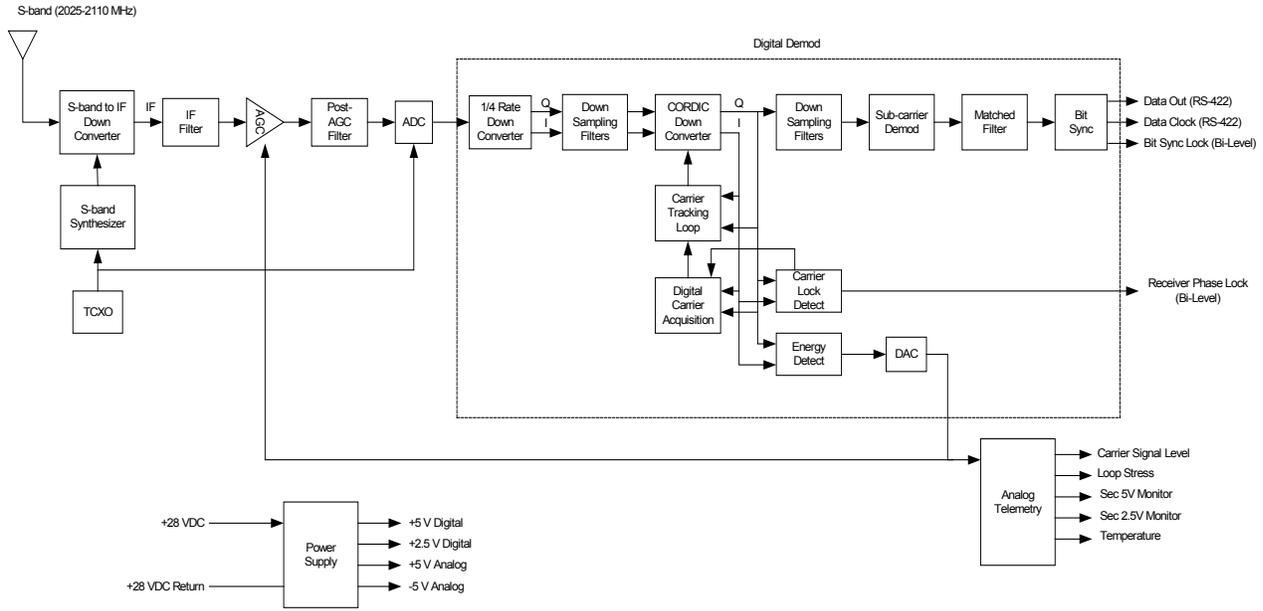
**Figure 1.** STDN Digital Receiver System-level Block Diagram
