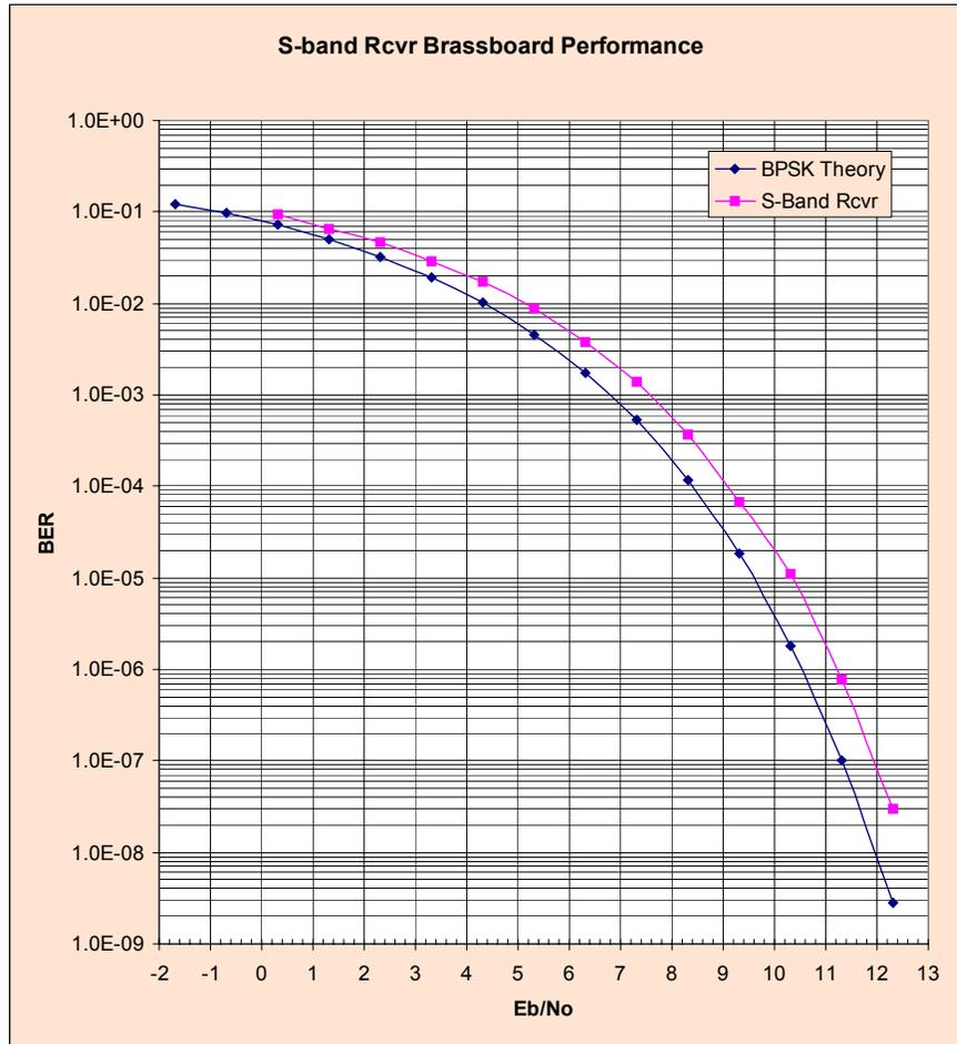
**Figure 8.** S-band Receiver Brassboard Error Probability vs. Eb/No
