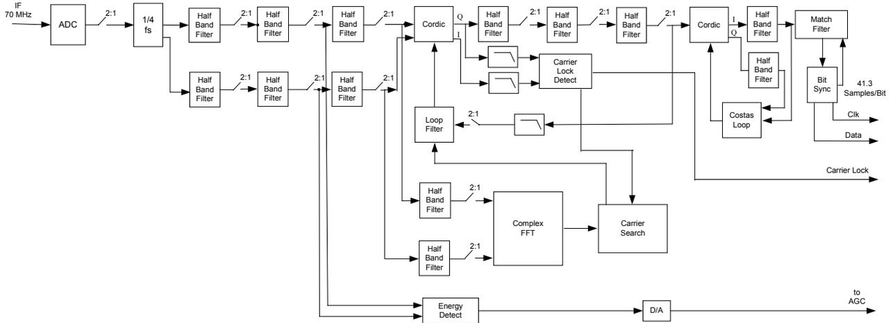
**Figure 3.** Digital Demodulator Functional Block Diagram
