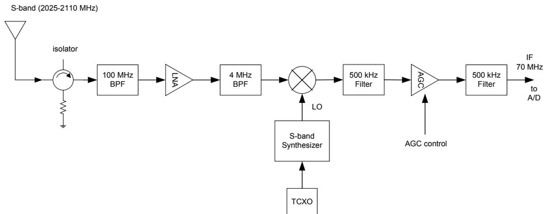
**Figure 2.** RF/IF Functional Block Diagram
