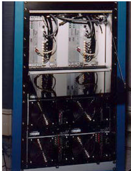
Figure 2. Two ACD Card Sets with Redundant, Hot-swappable Power
