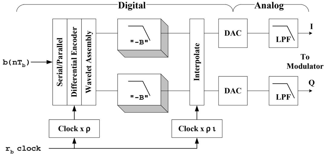
**Figure 1:** Baseband signal generator example.
