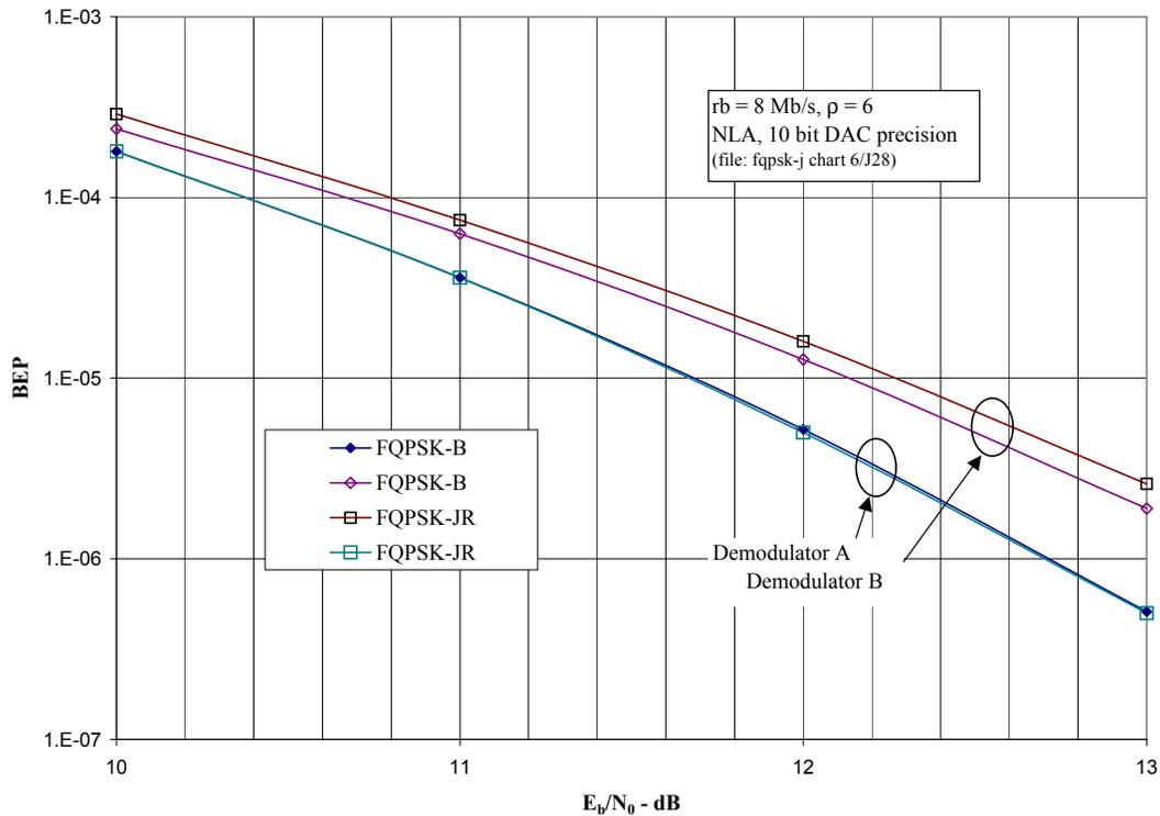
**Figure 9:** AWGN detection performance, hard decision detectors, differential encoding.
