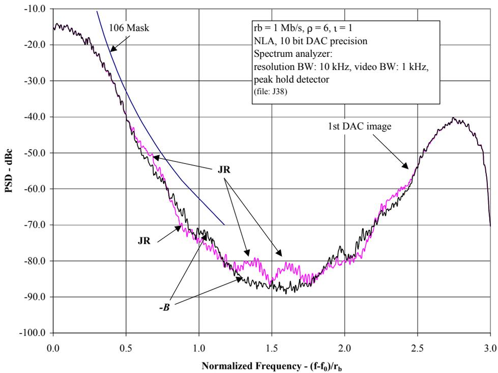
Figure 5: JR versus  $-B$  baseline PSD, no interpolation, no image filter.
