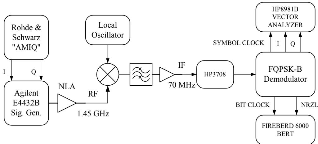
**Figure 3:** Test equipment.
