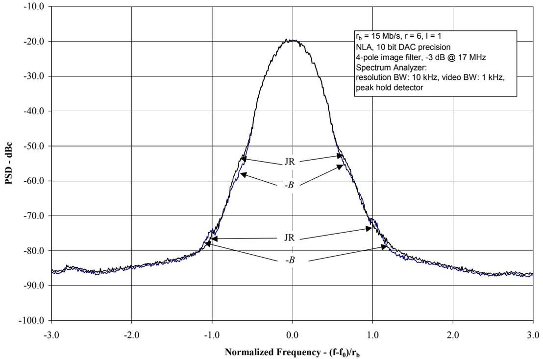
**Figure 10:** Example of complete JR and  $-B$  RF spectra with image filter and NLA.
