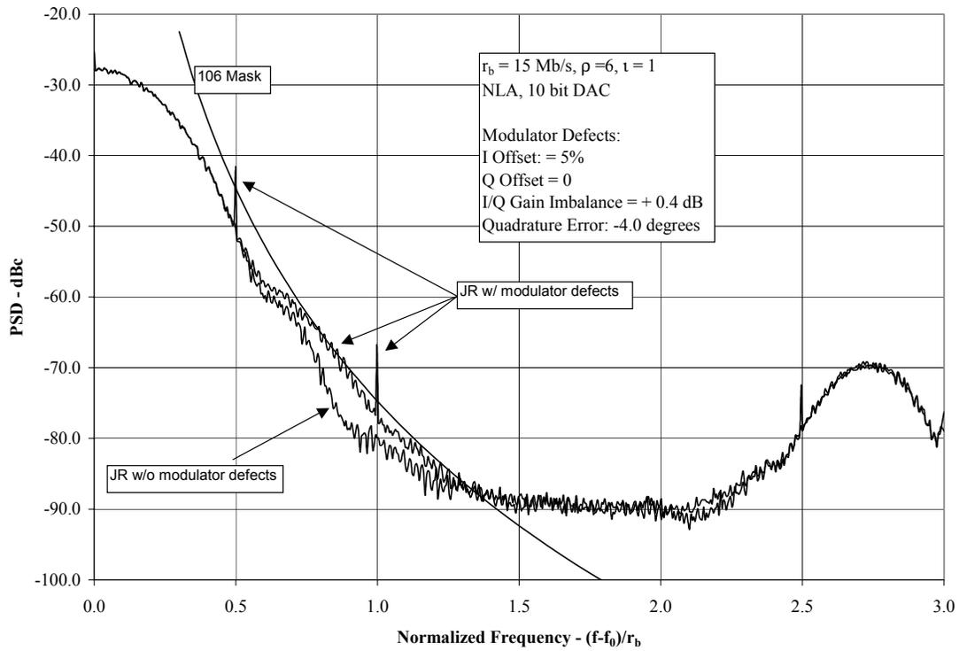
**Figure 8:** Example of I/Q modulator defect impact.
