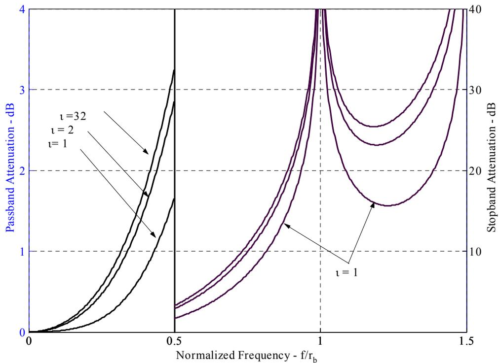
**Figure 4:** Solid lines are the JF frequency response. Broken lines are combined response of JF filter and 4-stage CIC filter at interpolation ratios of 2 and 32.
