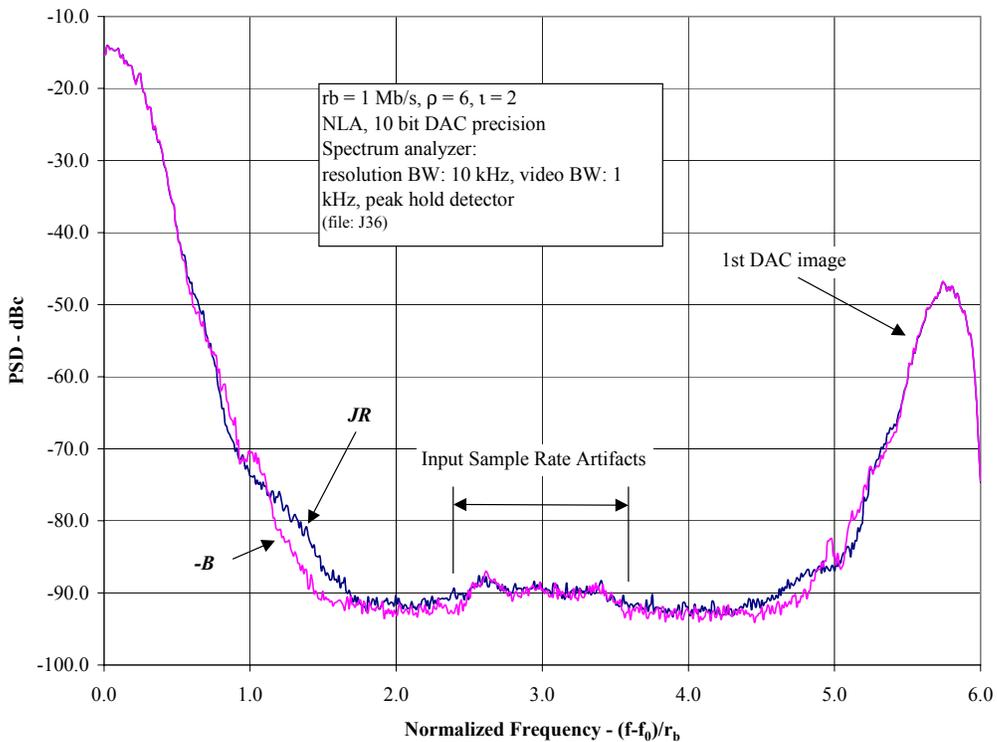
Figure 6: JR versus  $-B$  baseline PSD, with interpolation, no image filter.
