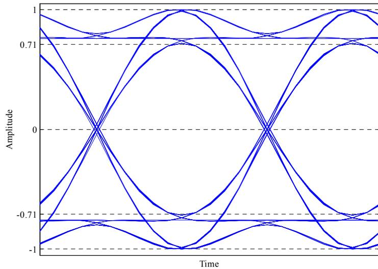
**Figure 11:** FQPSK-JR baseband generator eye diagram, I or Q channel,  $\tau = 2$ ,  $A = 0.73$ .
