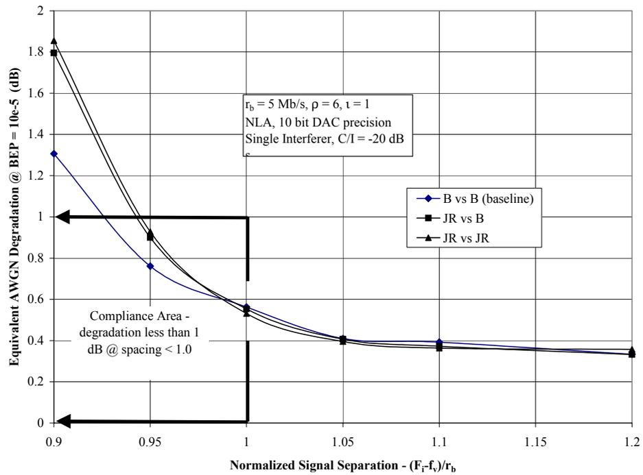
**Figure 7:** JR ACI performance with benchmark demodulator.
