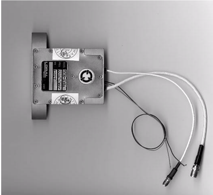
Figure 3. DTM - digital telemetry system
