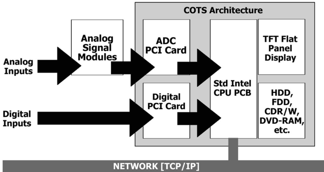
Figure 1 – Basic System Architecture
