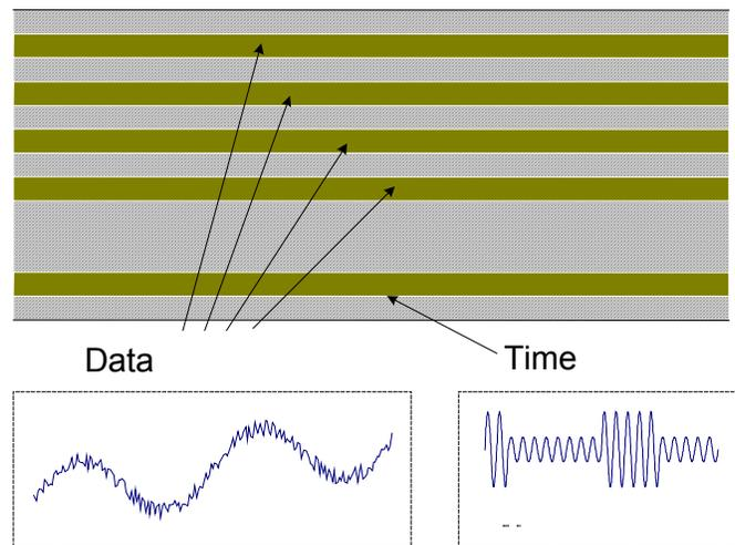
Digital recording techniques require a different method for keeping track of data synchronicity and timing. In this case, all data is first digitised, and then placed onto the media (still tape, solid state memory, optical or hard disc). The data block from different sources are placed on the media identified by their source ID in the packet header. The absolute time is placed also as one data block similarly.
