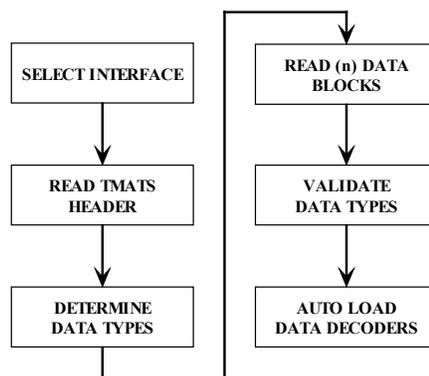
If the appropriate interfaces are present in the Windows OS environment the Solid State Memory modules containing the data can be presented as a drive volume in the Windows shell. Utilizing registered Component Object Module (COM) objects the data can be decoded and processed on the
