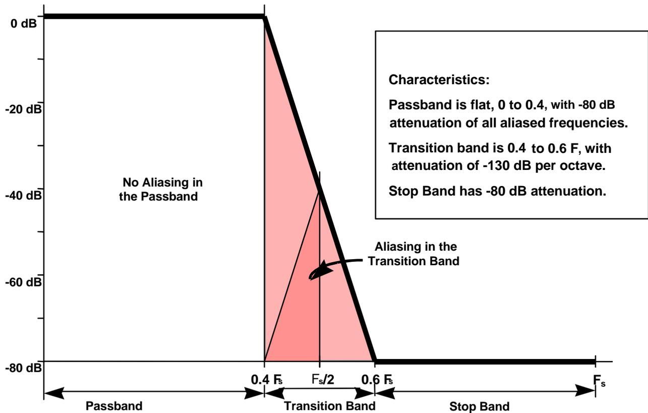
**Figure 2. Low-Pass Filter Without Aliasing in the Passband**
