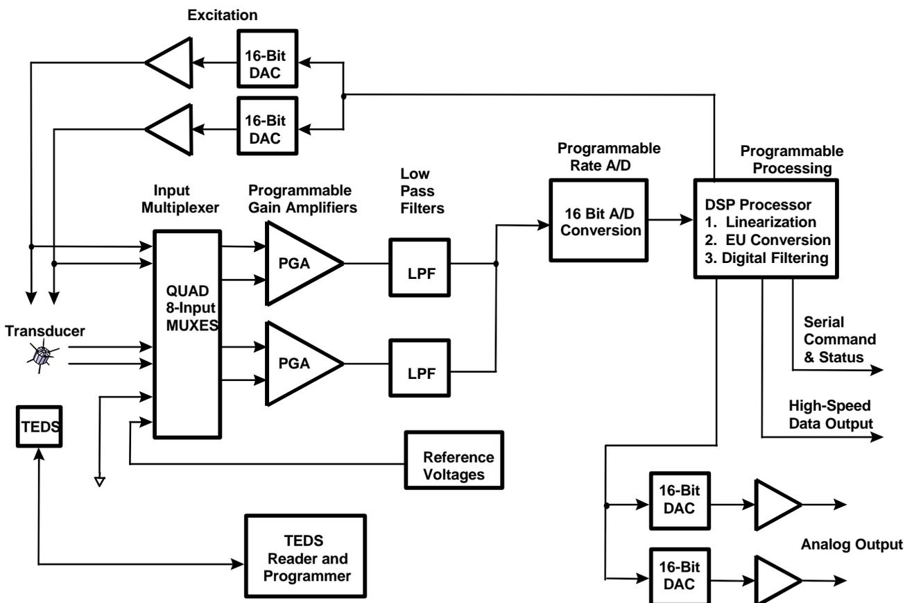
**Figure 1. USCA Block Diagram**
