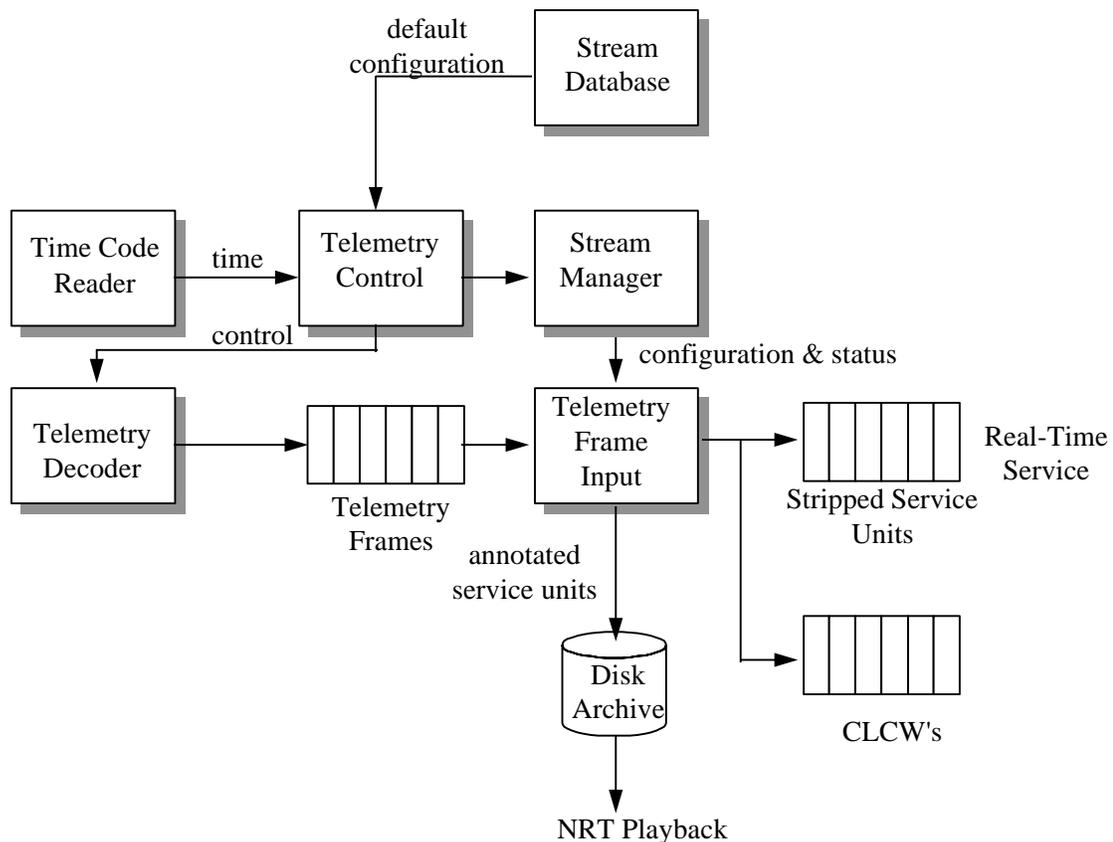
**Figure 4 Telemetry Control**
