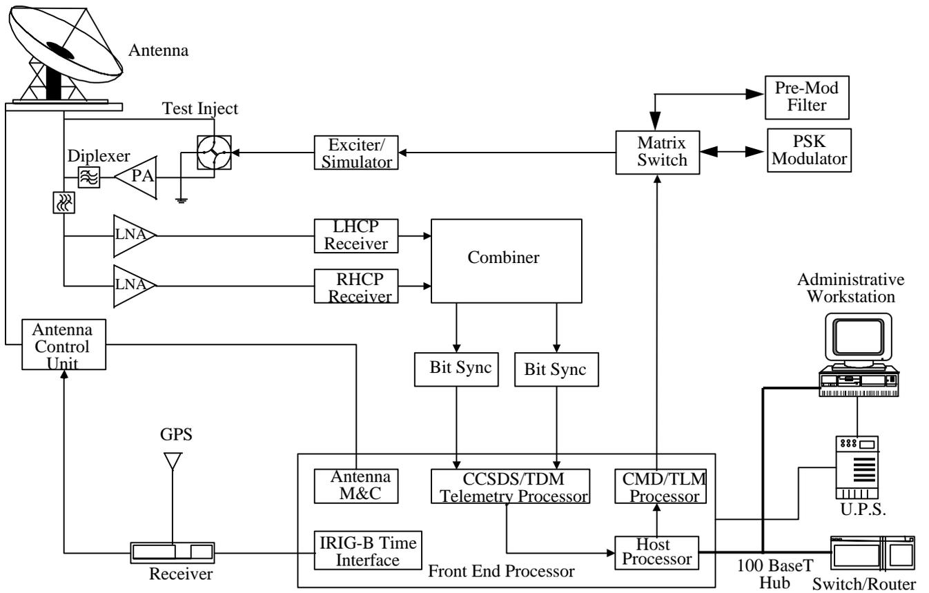
**FIGURE 1 LEO-T High Level Block Diagram**
