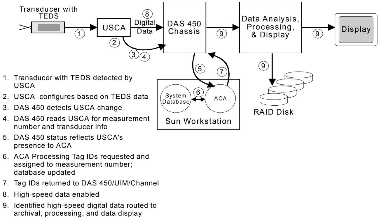
Figure 6. Automated Setup Data Flow with New Measurement
