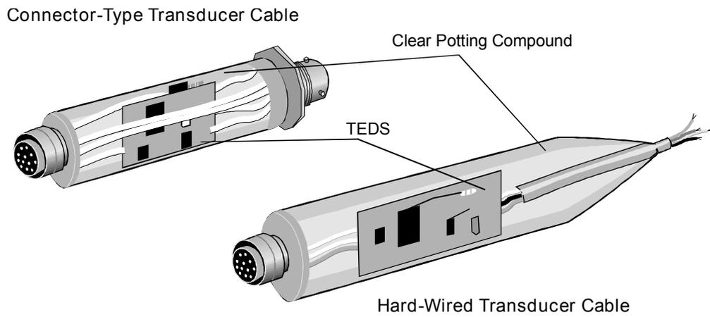
Figure 2B. Encapsulated TEDS in Clear Potting Compound
