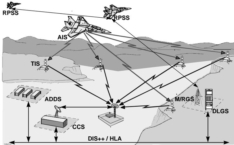
**Figure 8: Integrated Test and Training Instrumentation Architecture**
