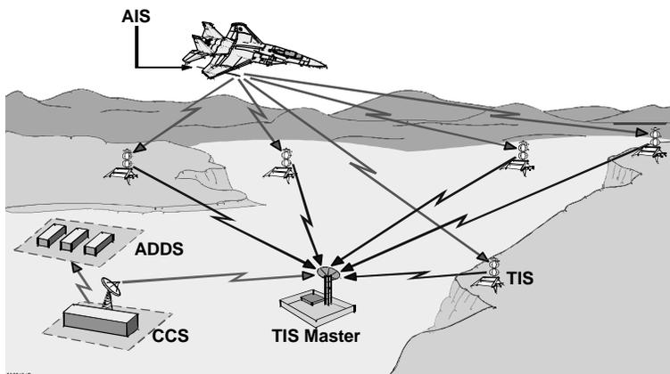
**Figure 4: ACTS Multilateration Instrumentation**
