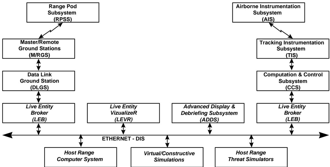
**Figure 7: Integrated Test and Training Instrumentation Architecture**
