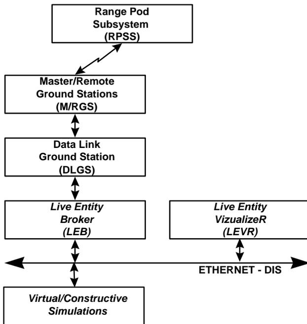
**Figure 5: DIS-Compatible Test Instrumentation Architecture**
