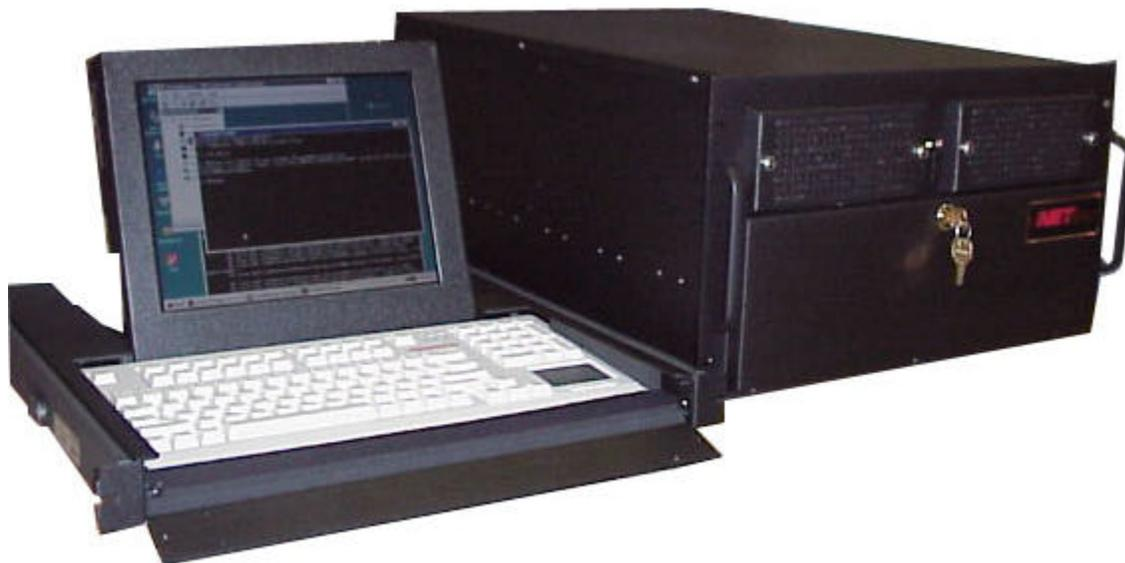
**Figure 4. Rack-Mount TT&C System Chassis with Flip-Up Display**
