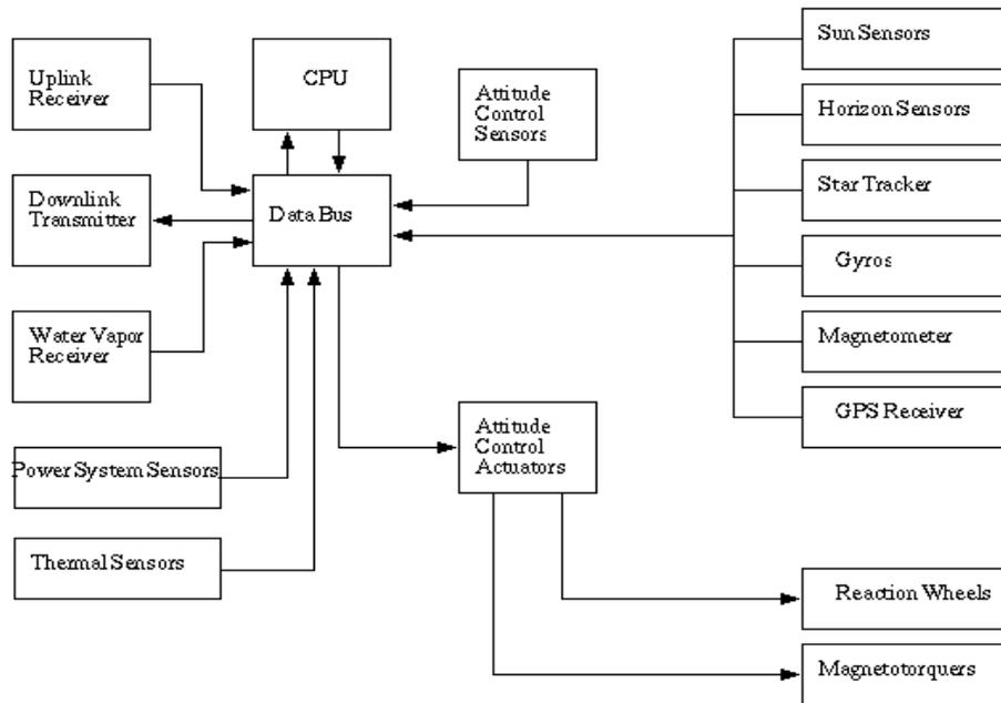
Fig. 1. Satellite Block Diagram
