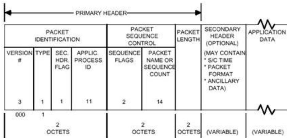
Fig. 3. Command Packet Structure
