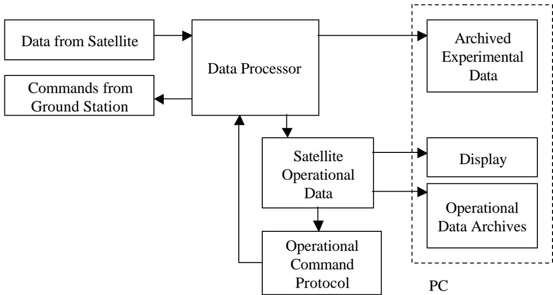
Fig. 6. Major Components of Ground Station CPU.
