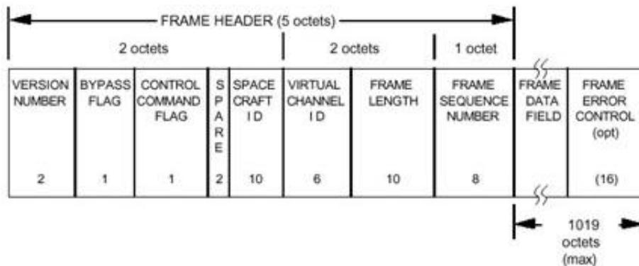
Fig. 4. Telecommand Transfer Frame
