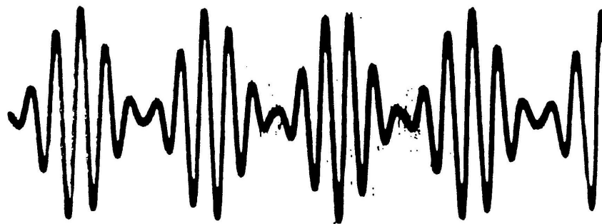
Oscilloscope trace of 89 Hz sine wave modulation of 480 Hz sine wave carrier Figure 4
