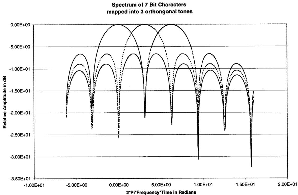
Figure 5 Normalized RF Spectrum of three adjacent tones
