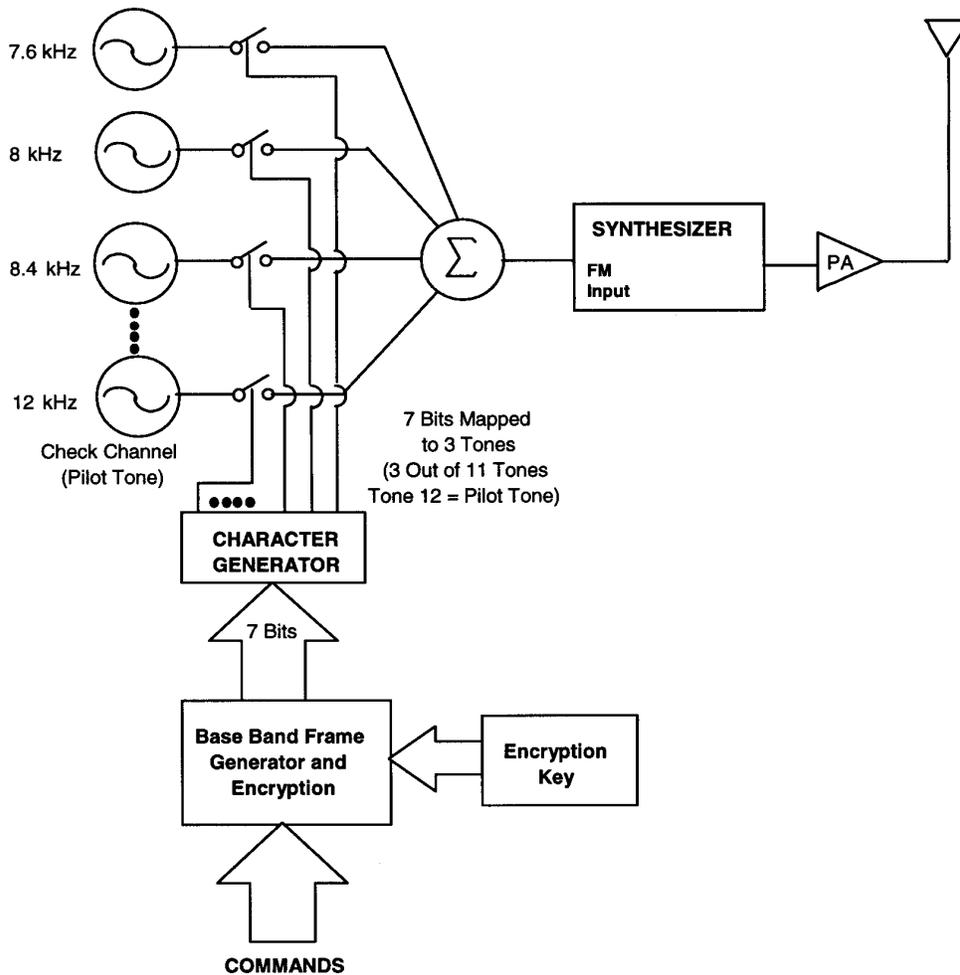
**Figure 1: Enhanced Flight Termination System Transmitter**
