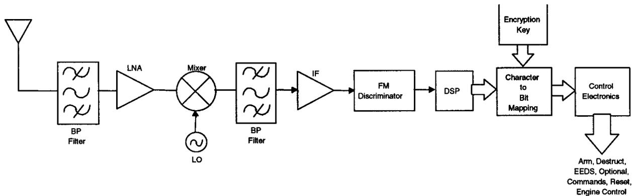
**Figure 2: Enhanced Flight Termination System Receiver.**
