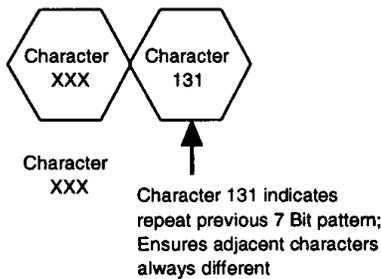
**Figure 3 Base band message frame format for the High Alphabet based system.**
