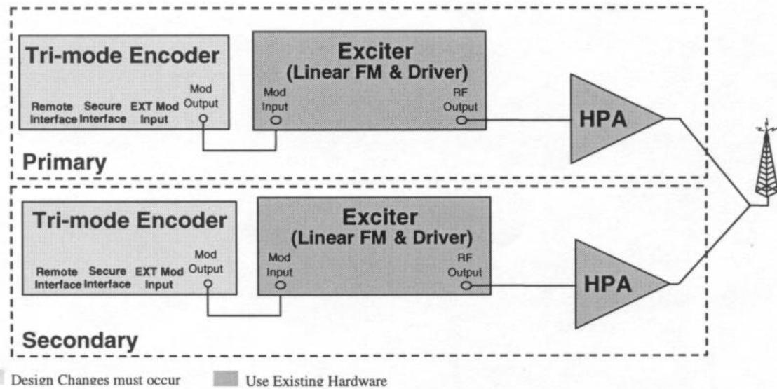
**Figure 1-1 Block Diagram Of Existing System Modifications Required**
