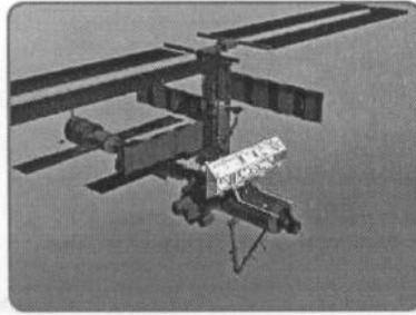
**Flight 8A** delivers the center segment of the 300-foot truss that will be attached to the U.S. Lab; 2001.
