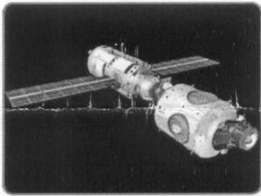
**Flight 2A** launched Node 1 (Unity) with mating adapters that connect US and Russian elements and provided a Shuttle docking location; 2000.
