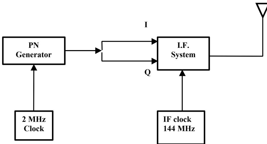
Figure 2. VHF Transmitter Test-bed
