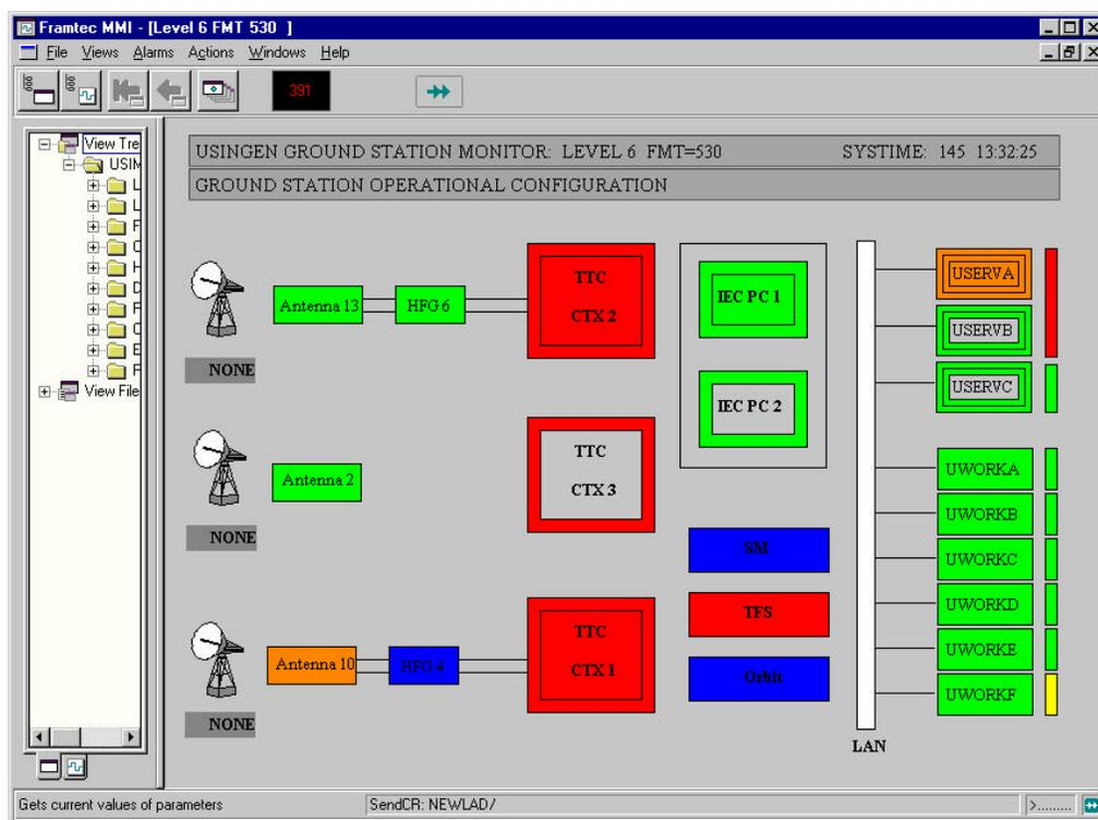
Figure 4. Typical display “system overview” (in emergency state)
