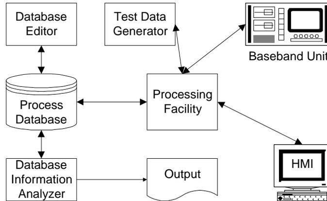
Figure 4: Components of FRAMTEC
