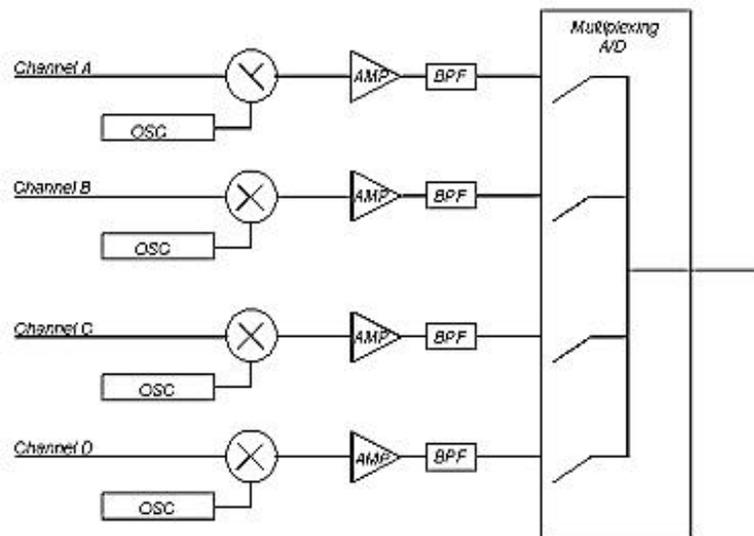
Figure 1: Science Receiver Functional Diagram
