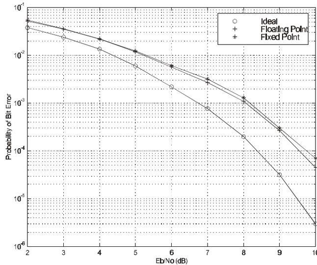
Figure 10. Demodulation Performance of the High Rate Parallel Receiver with FQPSK
