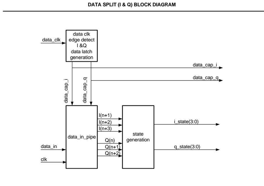
Figure 6. Serial Data Input and State Generation for Waveform Selection
