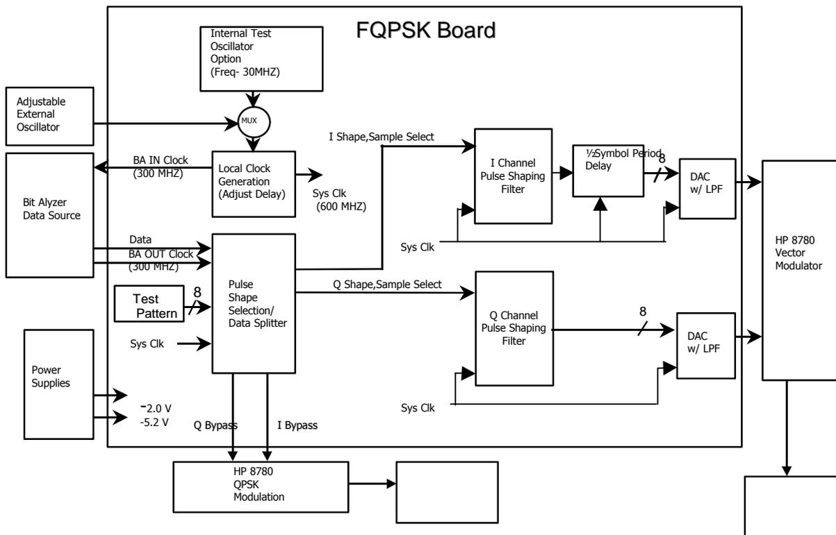
Figure 3. NASA/GSFC FQPSK Modulator
