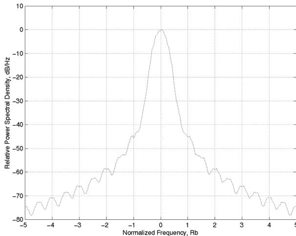
Figure 2. FQPSK Spectrum
