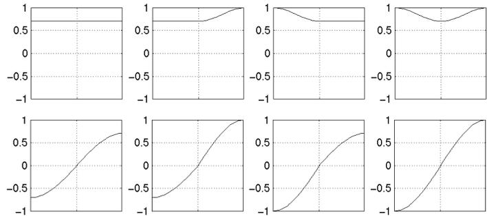
Figure 1. FQPSK waveforms
