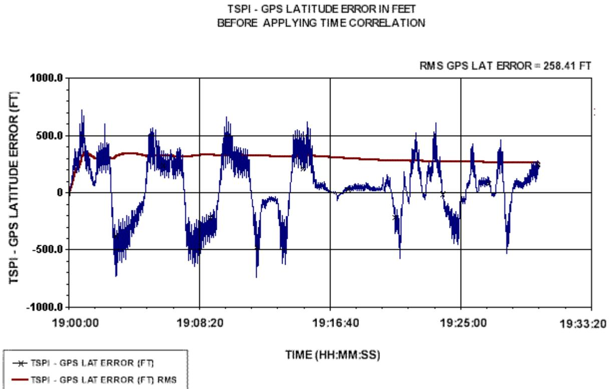
**Figure 1. GPS Latitude Error prior to time alignment software**
