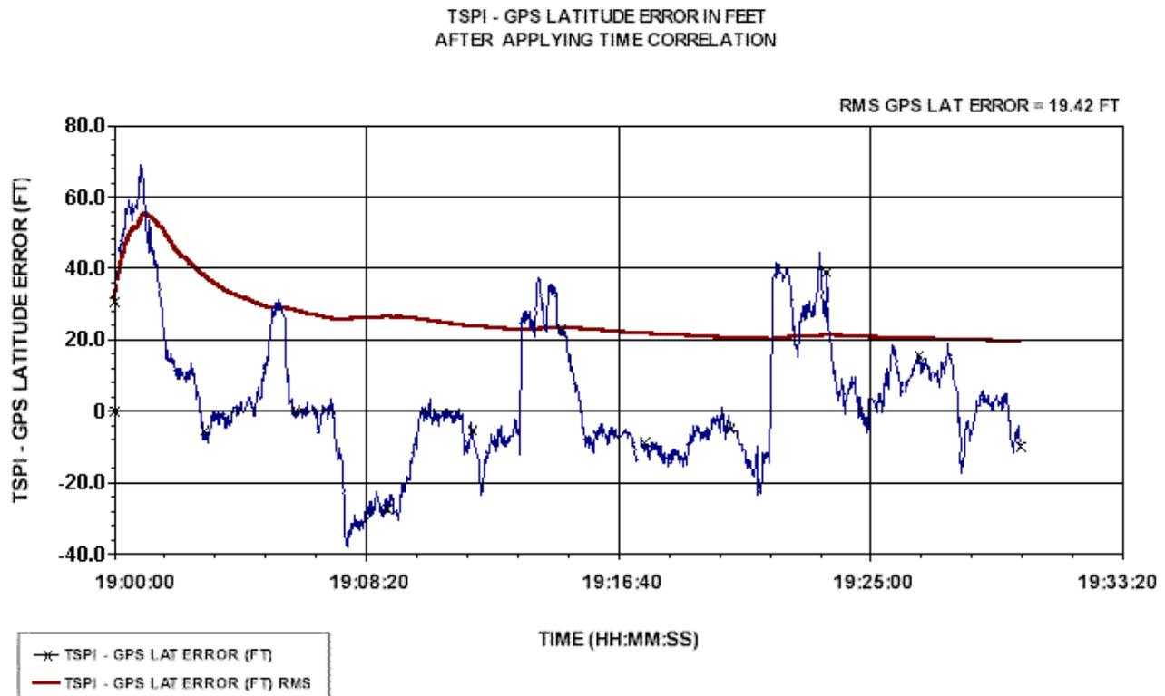
**Figure 2. GPS Latitude Error following time alignment software**
