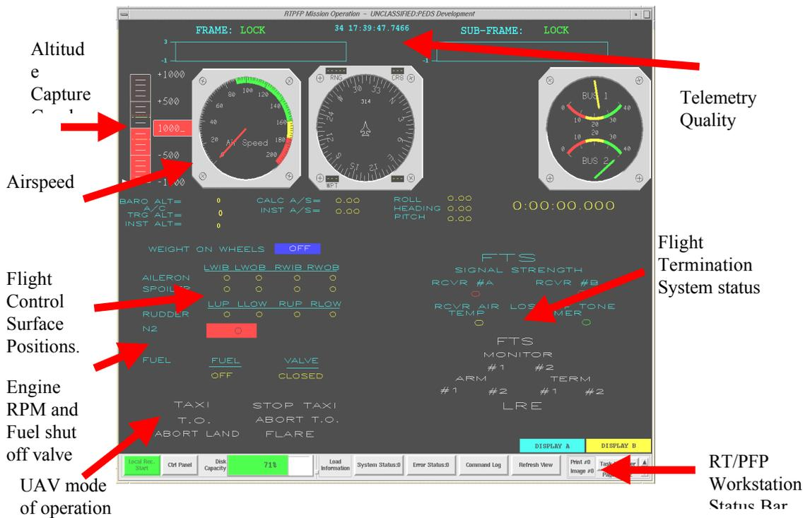
**RT/PFP Typical Range Safety UAV Telemetry Display**
