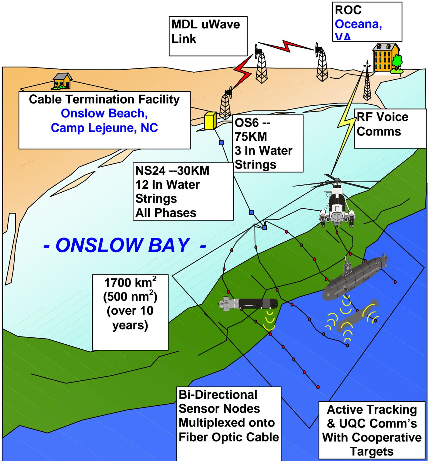
Figure 1 – EC SWTR System Configuration
