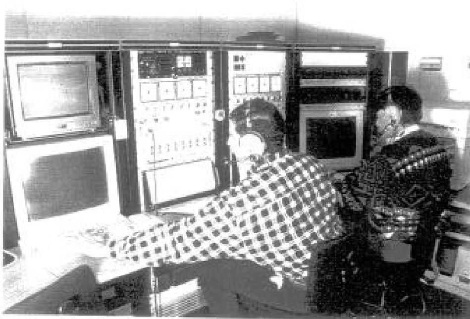
Ground telemetry control station. Data display in digital, analogue and brush recorder format as per requirement. (Photo: TFDC photographic section)
