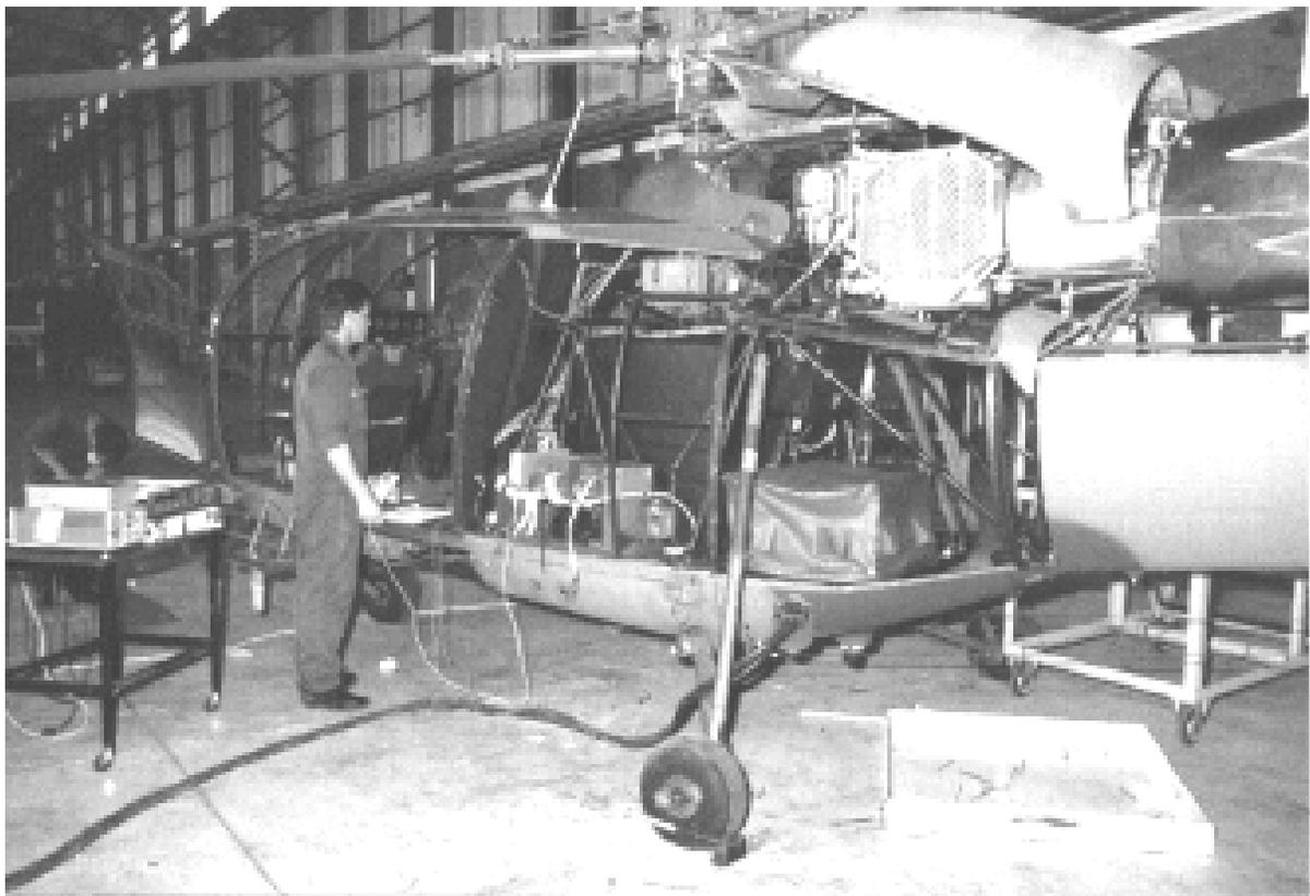
TFDC flight test instrumentation personnel busy fitting a SAAF Alouette III with a telemetry strap-on pack for low rotor RPM flight trials. (Photo: TFDC photo section)
