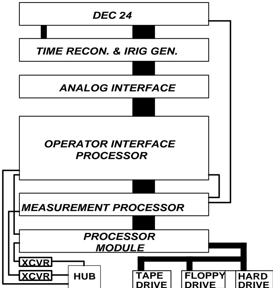
Figure 3 - Production Monitor Block Diagram
