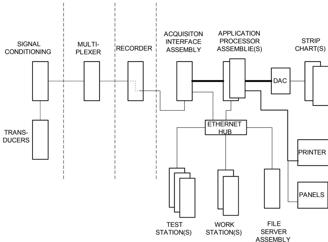
Figure 1- CFTDS Block Diagram
