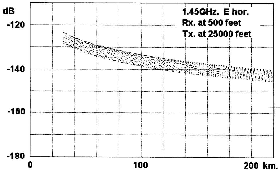
Fig. 3. Signal Variation Due to Multipath With 30% Reflection.
