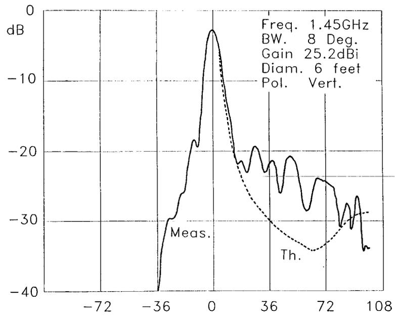
Fig. 6. Elevation Plot of Augustin/Sullivan Antenna
