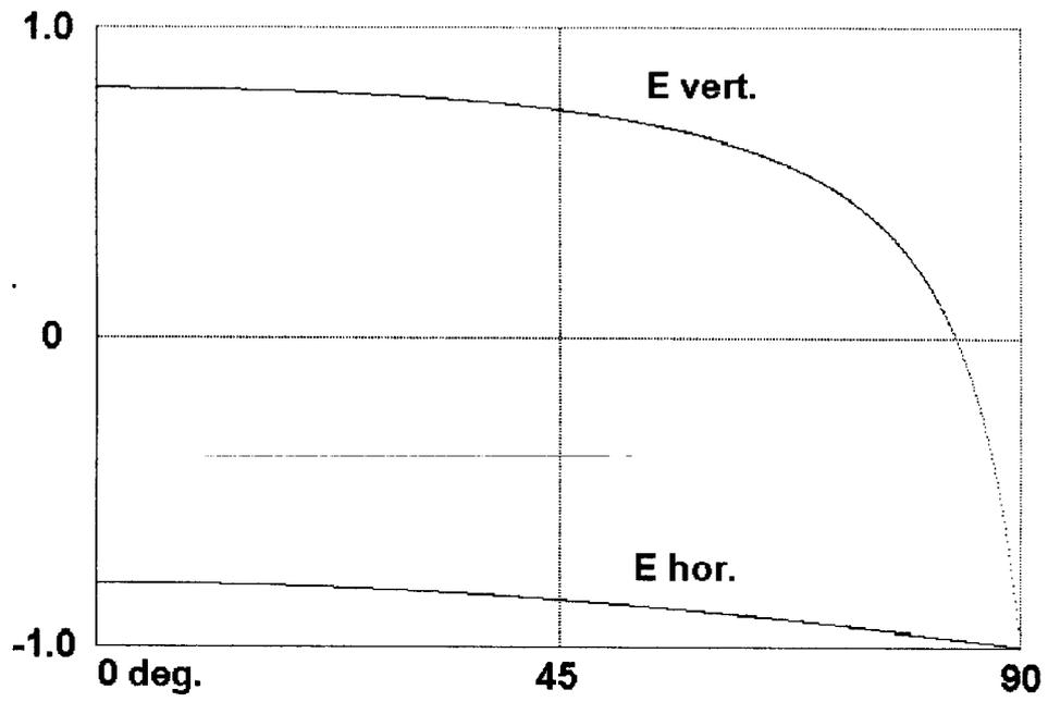
Fig. 1. Reflection Coefficient of Calm Sea at 1.45GHz.
