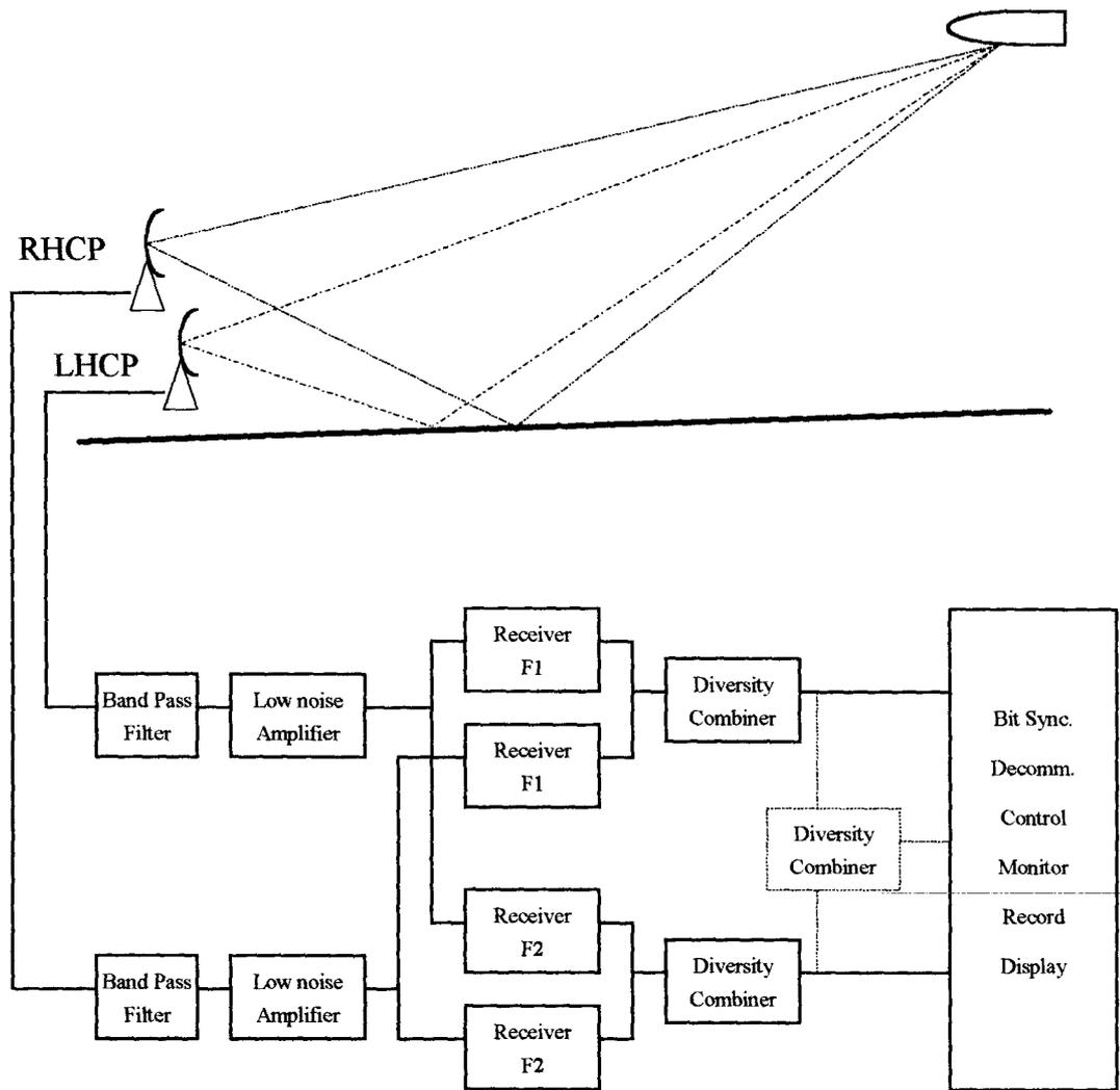
Fig. 5 System Block Diagram
