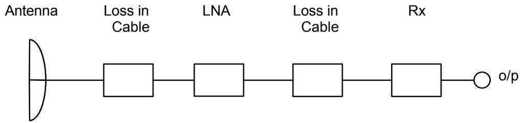
The effective noise present at the LNA input is considered in two parts; noise originating from items prior to this point, and noise originating from subsequent items. For the system as a whole bandwidth is constant so that the noise power can be normalised to absolute temperature which can then be summed arithmetically.
