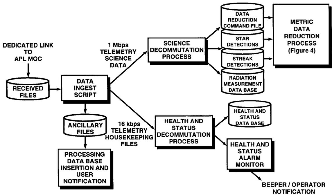
Figure 3. Processing applied to incoming telemetry files
