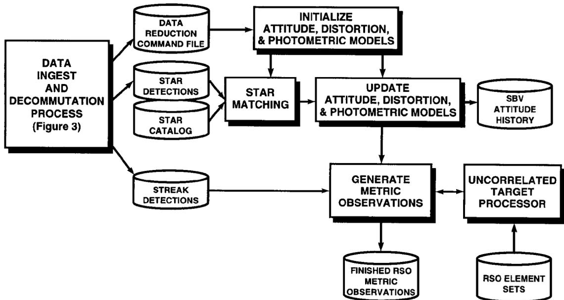
Figure 4. Processing applied to SBV metric data
